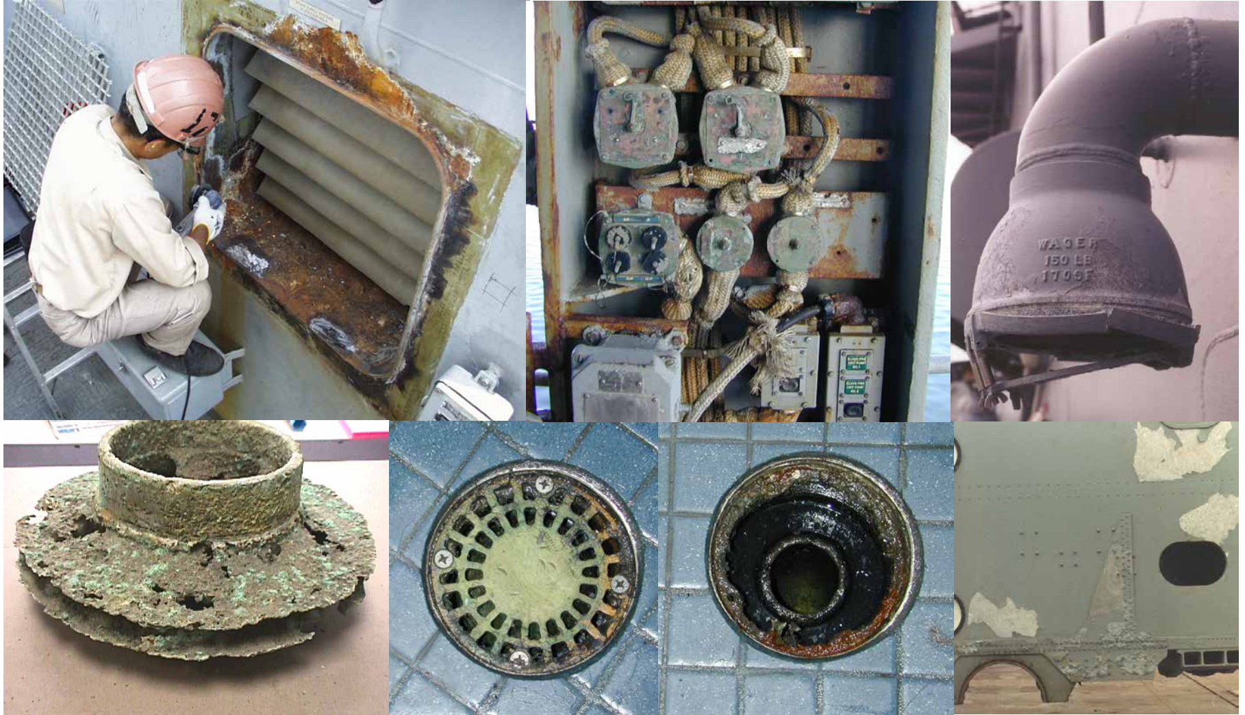
Examples of Corroded Metal Components on Navy Ships [Jeff Goldring, NAVSEA 05P24 and Eric Greene]
