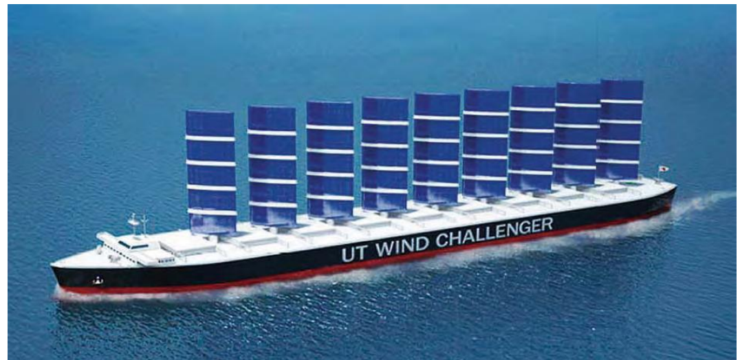
Proposed cargo ship with telescopically reefing hard composite sails [Kazuyuki Ouchi and Kiyoshi Uzawa of the University of Tokyo, Japan]
