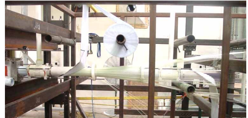
Glass rod, felt and polyurethane fabricated by pultrusion
