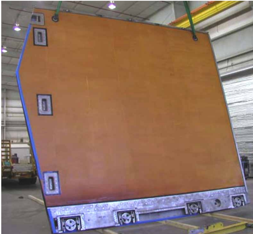
Helicopter hanger door developed by Seemann Composites in 2000
