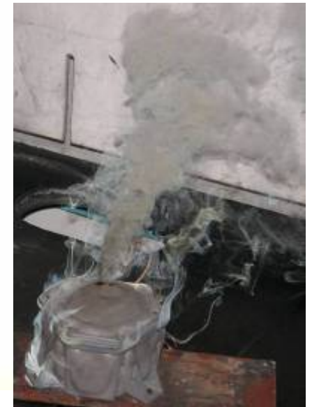
Fire Test of Glenair Modar Electrical Box
