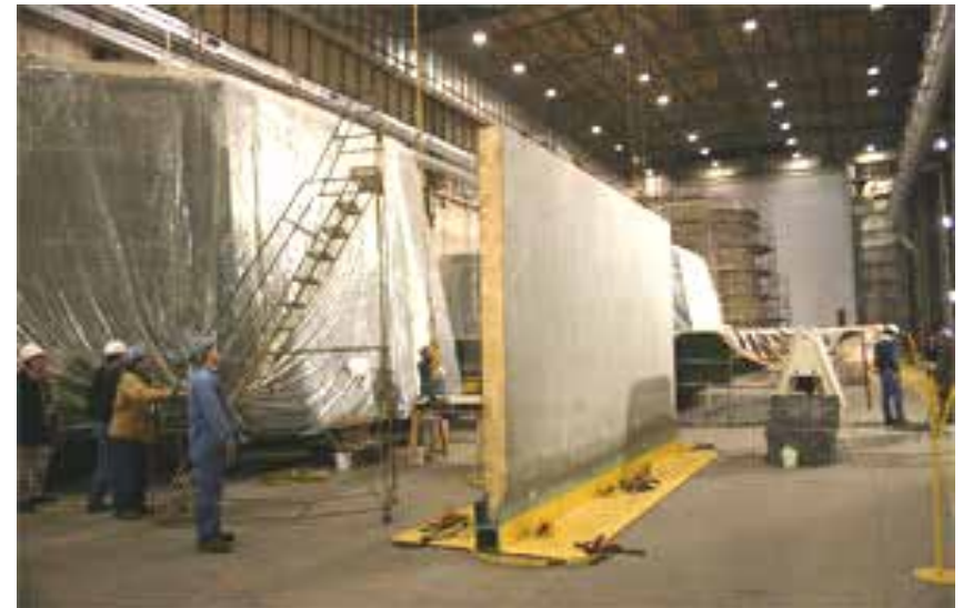
Composite deckhouse to steel deck joint R & D program by the ONR ManTech program
