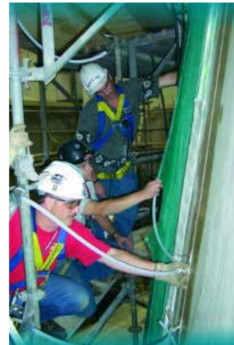
LPD 17 AEM/S Seam 40-foot Vertical Infusion
