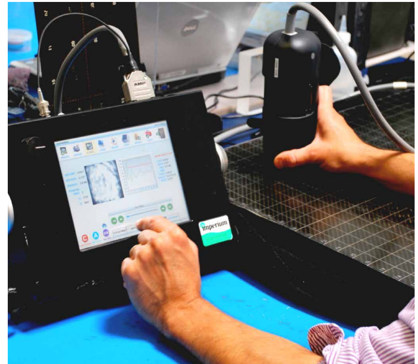
Imperium Acoustocam used to inspect test panel with simulated defects
