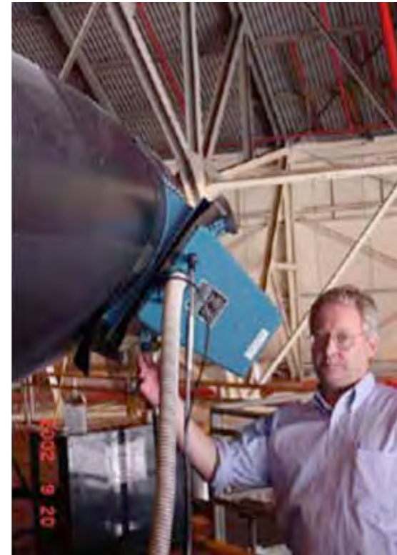
Shearography principal [Collrep 2006] and portable shearography device [Newman 2009]
