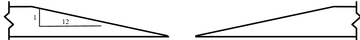
12:1 Tapered Scarf Through Thickness Damage
