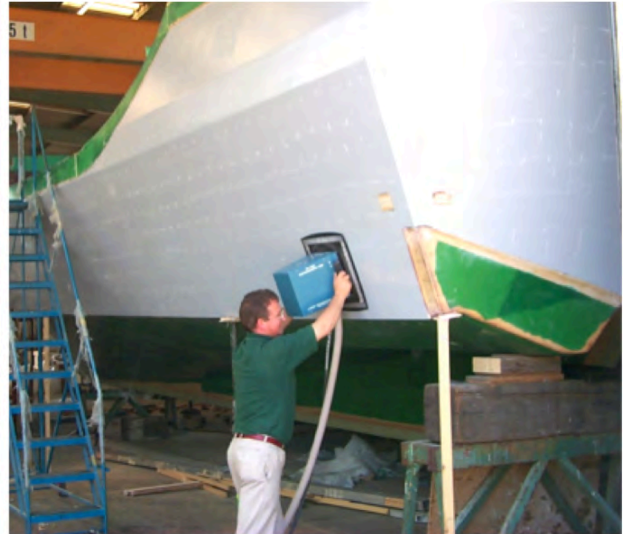
Laser shearography used to examine RNLI lifeboats [Laser Technology]
