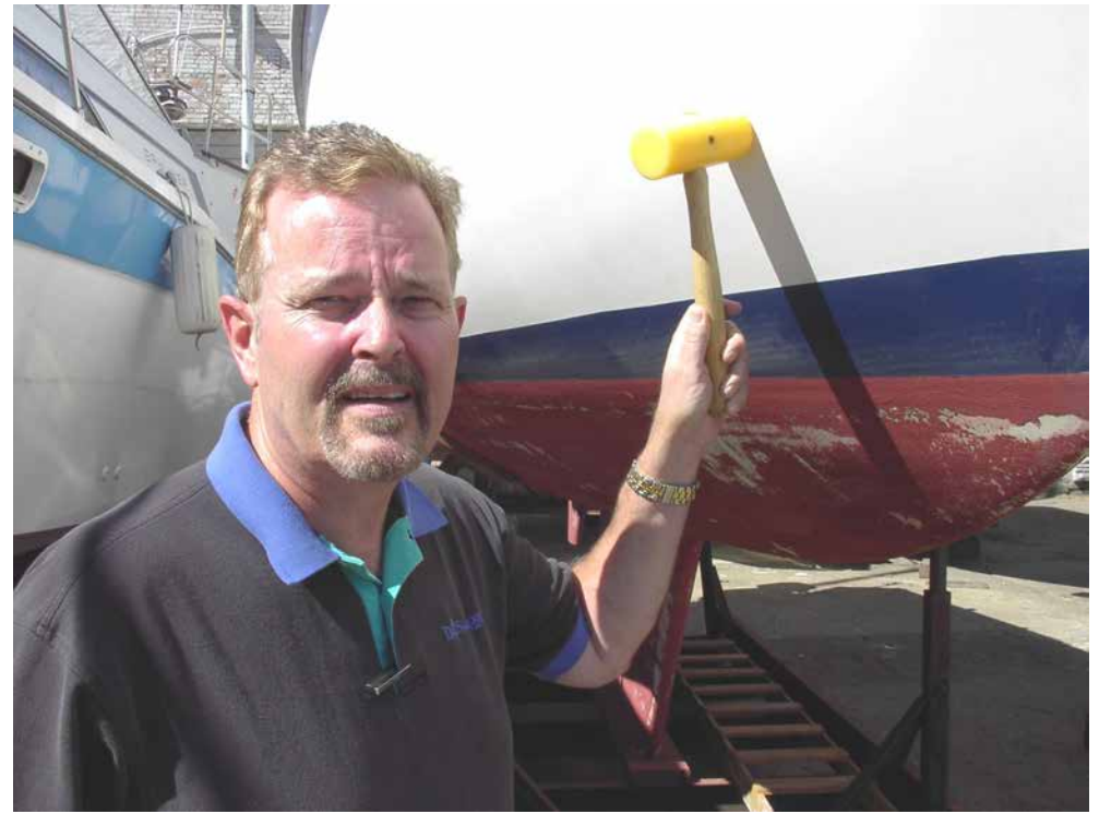
Marine surveyor Greg Davis uses sounding hammer on fiberglass boat hull
