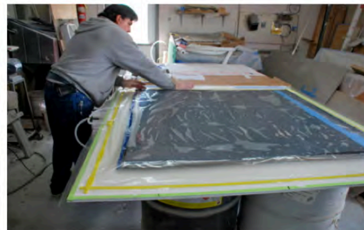
Vacuum bag is used to consolidate hand-laminated inner skin
