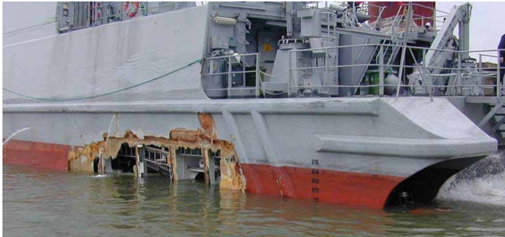
Mine Counter Measure Ship Collision with Dock
