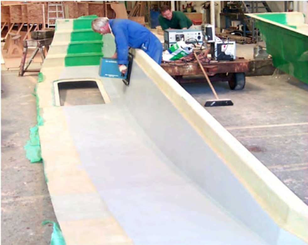
Laser shearography used to examine RNLI lifeboats [Laser Technology]
