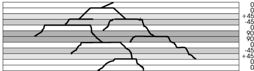
Pyramid Pattern Matrix Crack from impact.
