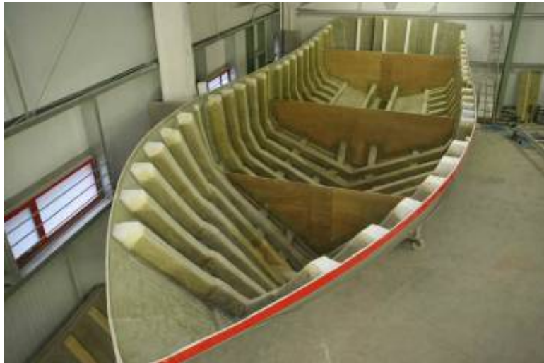
The hulls scantlings are very closely spaced @ 500mm centers giving a 4300mm panel width, the frames themselves are a huge 150 x 150mm resulting in a massively strong structure
