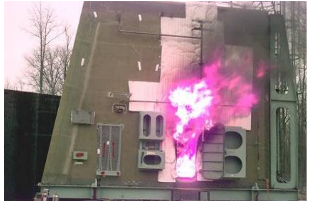
Full-Scale Fire Test for Helicopter Hanger Project with Fire Protection Around Door for Fire Test Only
