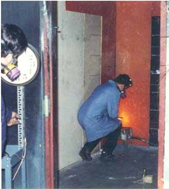
Lighting of Burner to Start Modified ISO 9705 Room Corner Test at VTEC Laboratories
