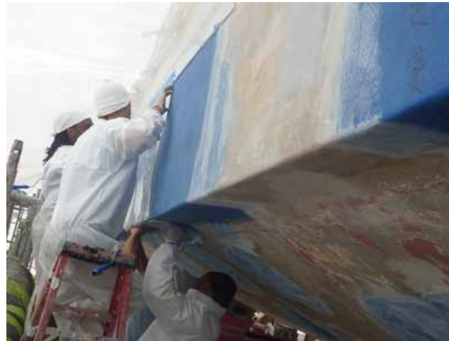
Waterline lamination in progress
