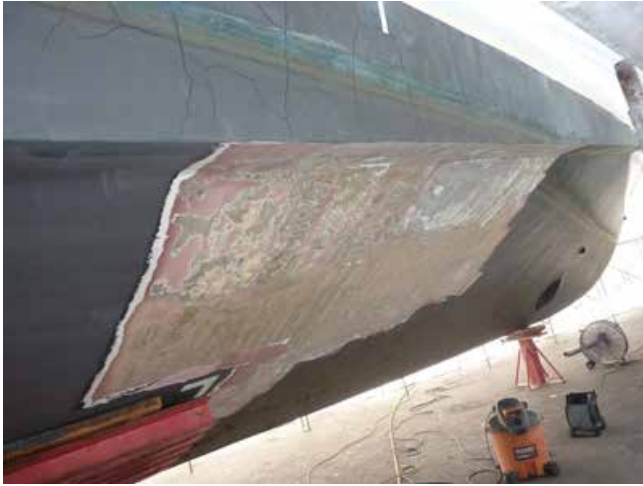
Peeling started on starboard side bow area, failed fairing, delamination and failed bottom paint
