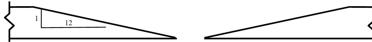
12:1 Tapered Scarf Through Thickness Damage
