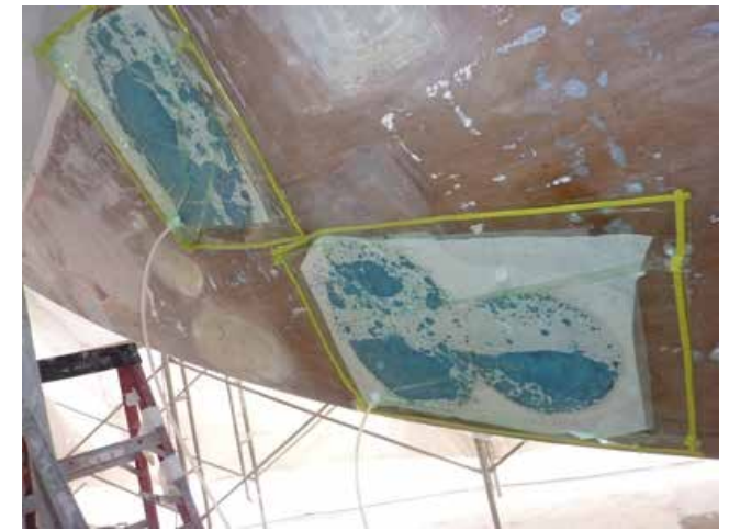
Using vacuum bags to consolidate repairs
