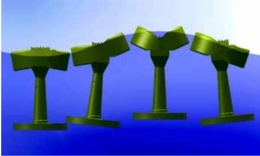
Energy is captured from both heave and surge motion
