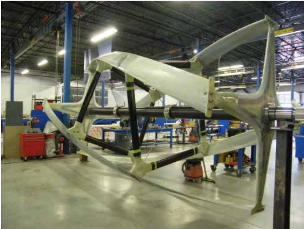
Helical turbine assembly built by Hall Spars for Ocean Renewable Power Company
