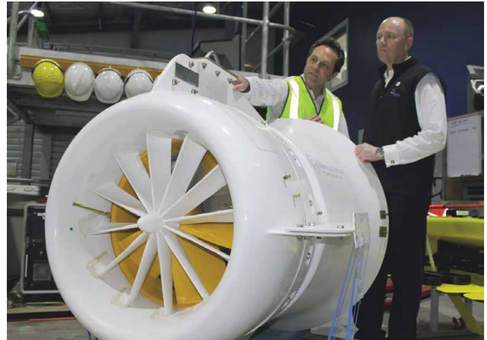
Michael Urch (left), and Darren Burrowes, inspecting a pre-production prototype of the 2 kW SeaUrchin.
