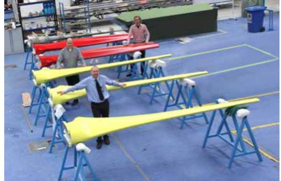
Airborne Marine in the Netherlands uses Resin Transfer Molding (RTM) injection technology in combination with preforming technology for turbine blades that will be installed at the EMEC test center in Orkney / Scotland.
