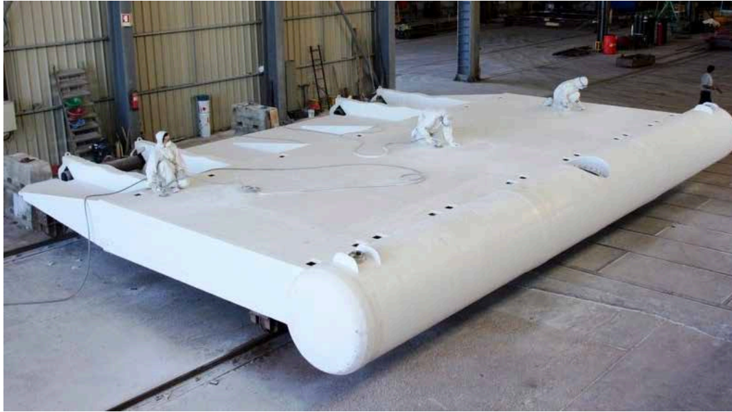
WaveRoller wave energy panel built with E-glass reinforcement
