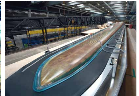
Laying up E-glass for vacuum resin infusion at LM Glasfiber
