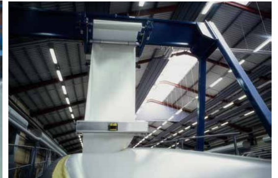
Laying up E-glass for vacuum resin infusion at LM Glasfiber
