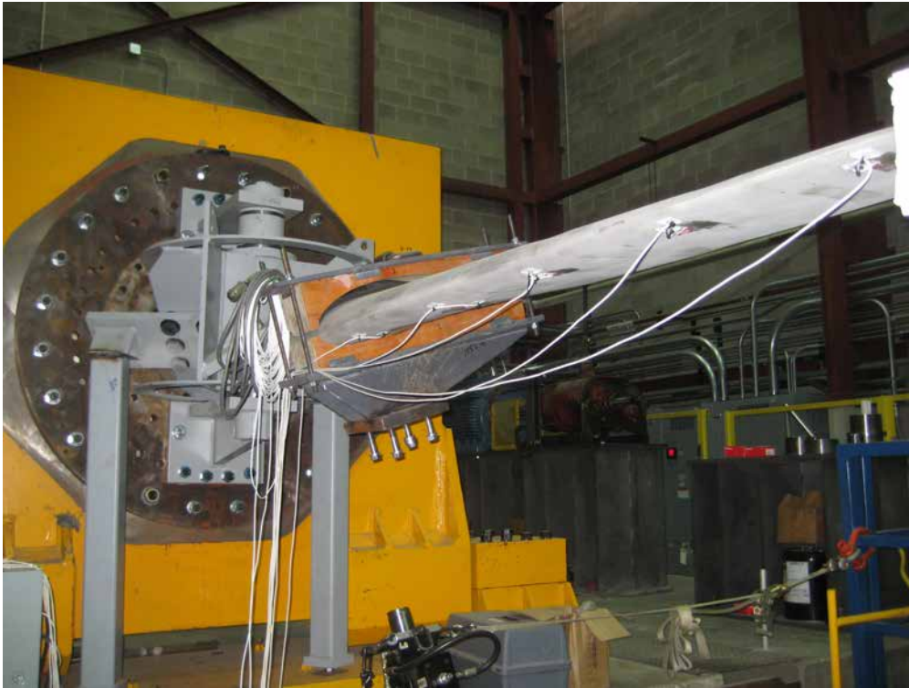
Water turbine blade being tested at the DoE National Renewable Energy Lab in Boulder, CO
