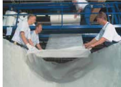
Laying up E-glass for vacuum resin infusion at LM Glasfiber
