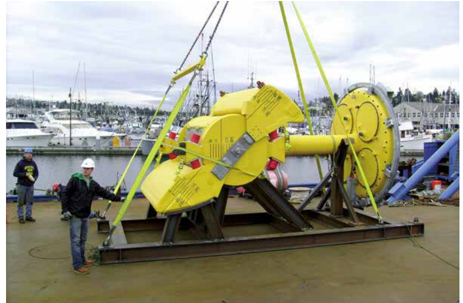
Energy is captured from both heave and surge motion
