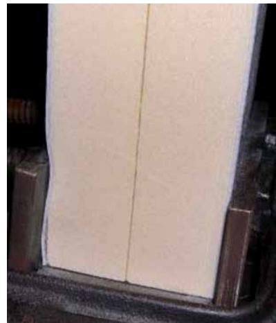
Local Face Buckling
