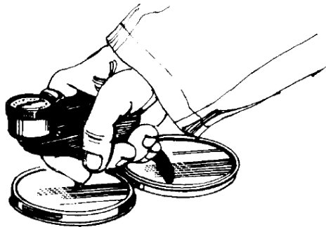
Barcol Impressor (Model 934 or 935 for readings over 75) [Cook, Polycor Polyester Gel Coats and Resins]
