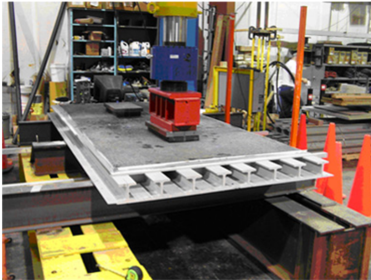
Florida DOT Lab Tested of ZellComp® 5-inch Composite Decking System for 2 million cycles
