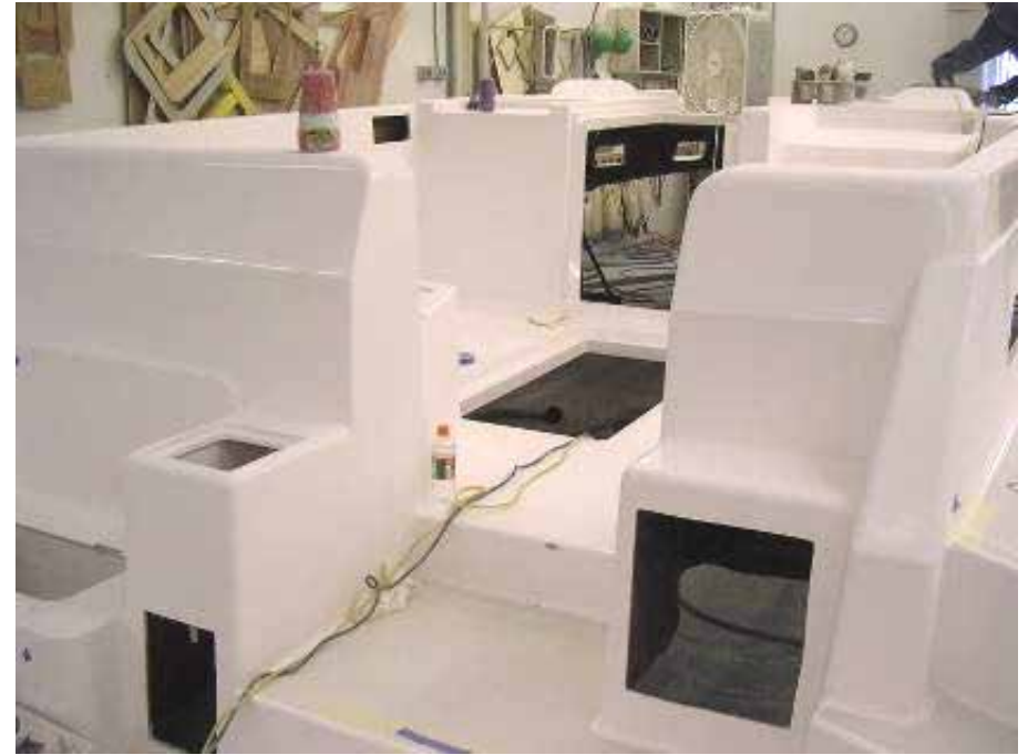
Production deck assembly built by Sabre Yachts
