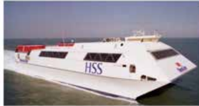
88 m aluminum high speed catamaran with an FRP composite superstructure
