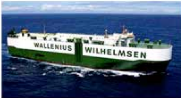
199 m RoRo vessel with an aluminum deck house
