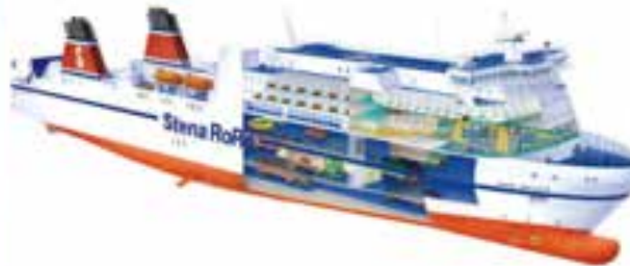
188 m RoPax vessel with an FRP composite superstructure
