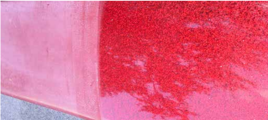
UV damaged (left) and restored gel coat (right)
