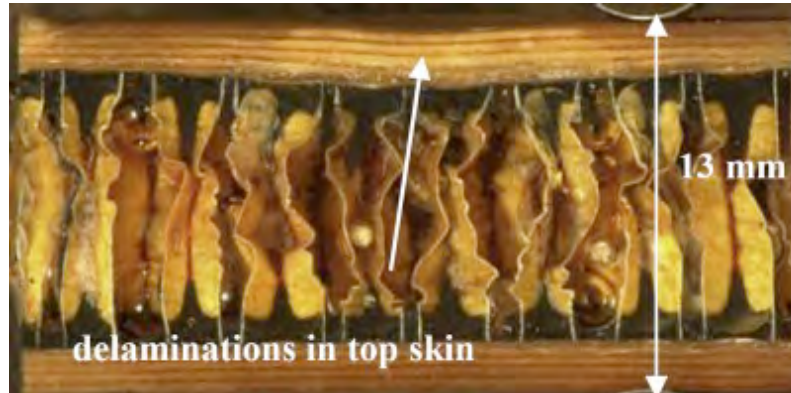
Digital photograph of impact delaminations in top skin of a sandwich construction
