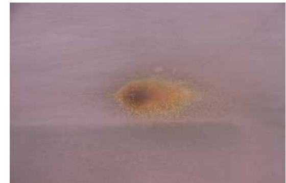
Lightning damage to carbon fiber yacht mast showing discharge path
