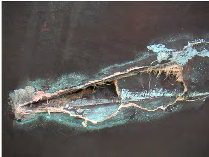
Roll stabilizer damaged after grounding (top) and resulting hull damage (below)
