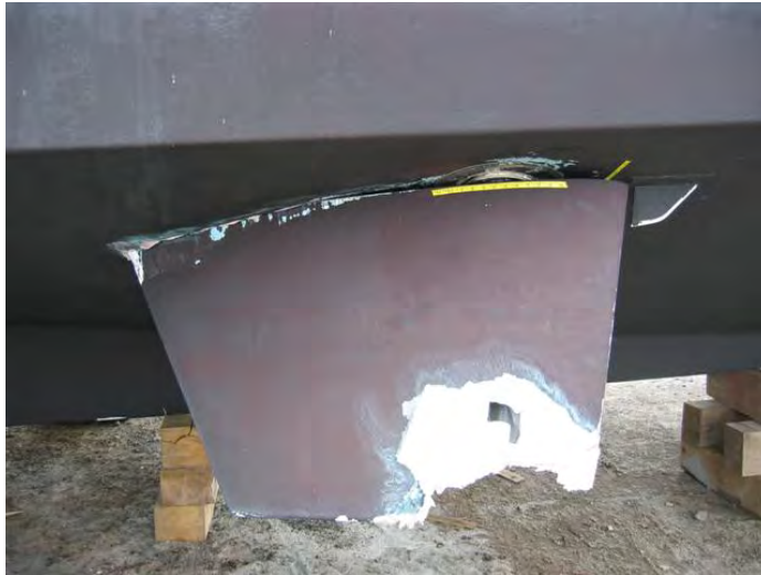
Roll stabilizer damaged after grounding (top) and resulting hull damage (below)
