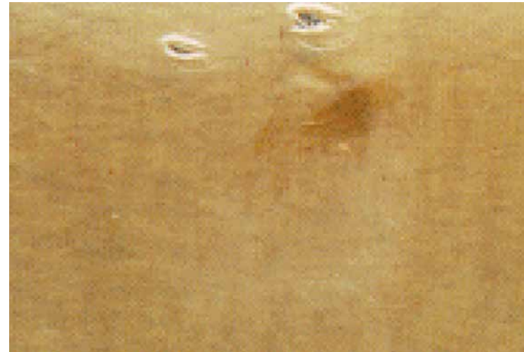
Fisheye Small globular mass that has not blended into surrounding material. Particularly evident in transparent or translucent materials
