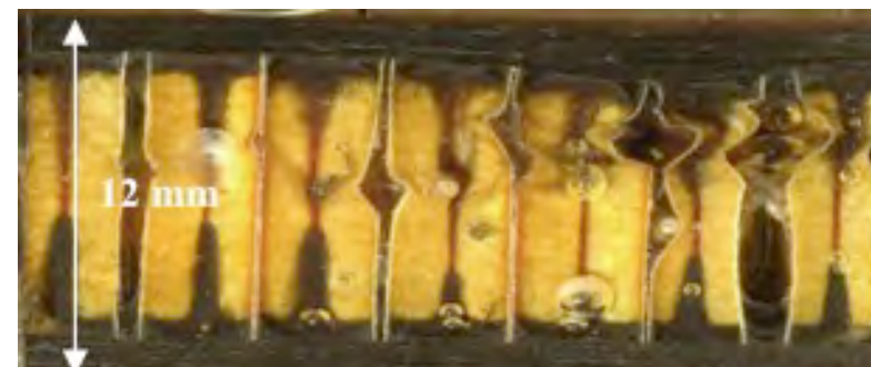
Digital photographs showing core crushing in (left) GRP-high density Nomex and (right) CFRP-medium density Nomex sandwich constructions
