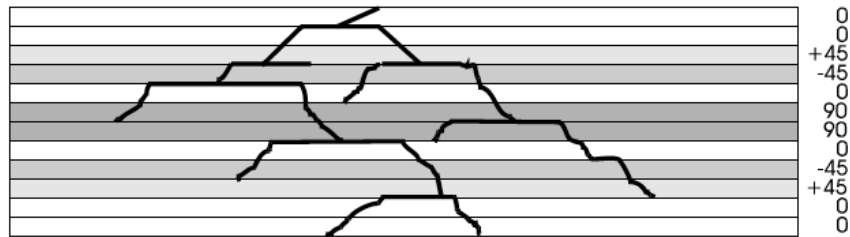
Pyramid Pattern Matrix Crack from impact.
