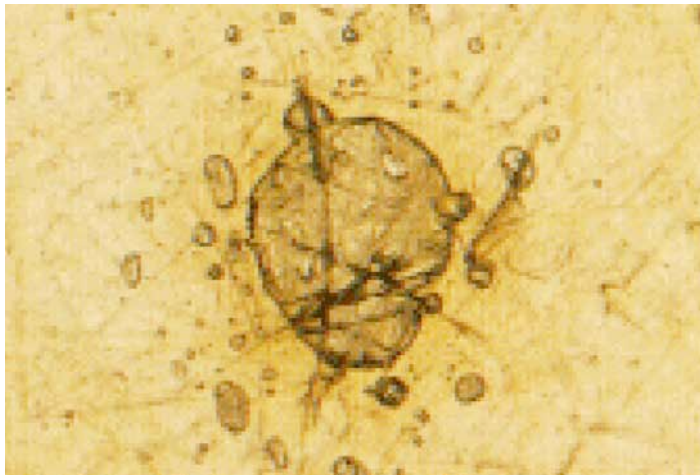
Worm hole Elongated void in surface or covered by thin film of cured resin.
