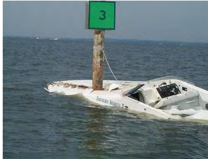
Just before 2 a.m., a 1992, 38-ft. Fountain power boat slammed into a fixed, channel marker, ripping a 17-ft. gash in the forward hull & becoming impaled on the steel piling holding the channel marker.
