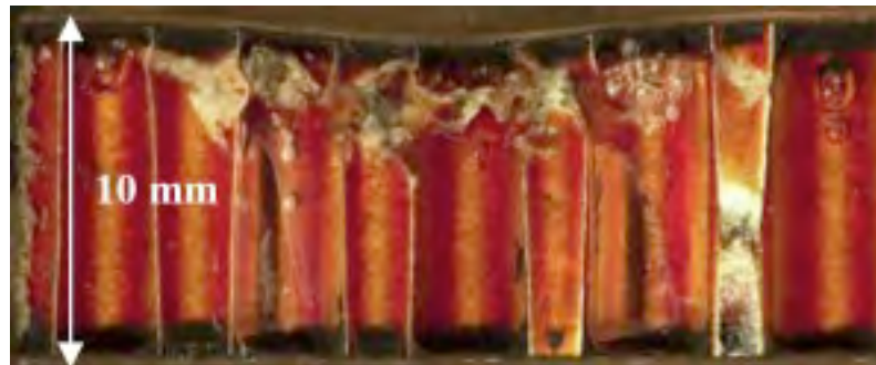
Digital photographs showing core crushing in (left) GRP-high density Nomex and (right) CFRP-medium density Nomex sandwich constructions
