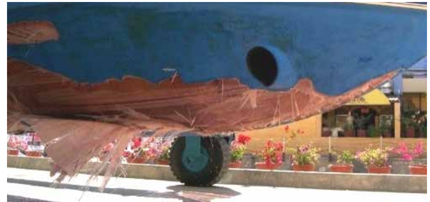
Damage to Viking 60 from Collision with Whale
