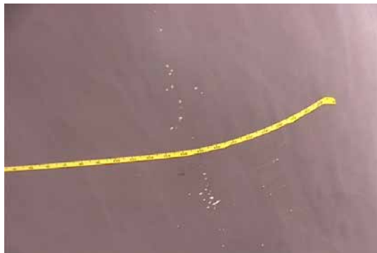
Lightning damage to carbon fiber yacht mast showing discharge path
