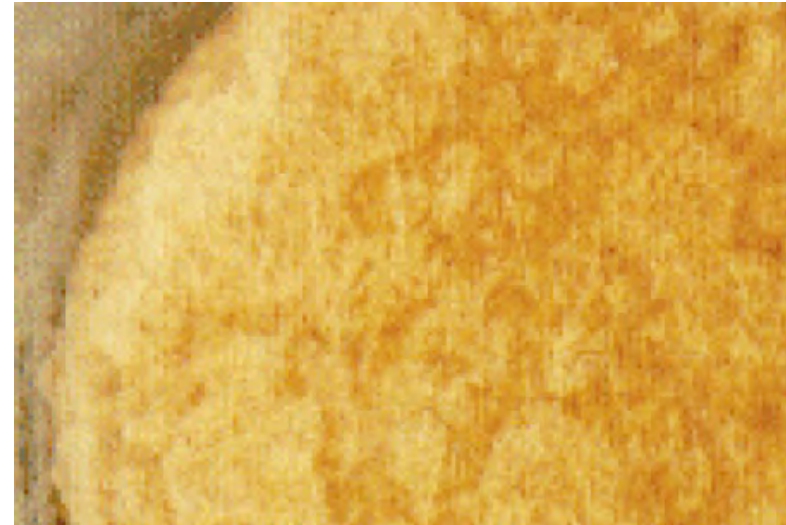
Blisters Rounded, sometimes sharply defined elevations of laminate surface resembling blisters.
