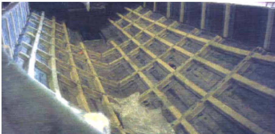
Norsafe lifeboat structural grid
