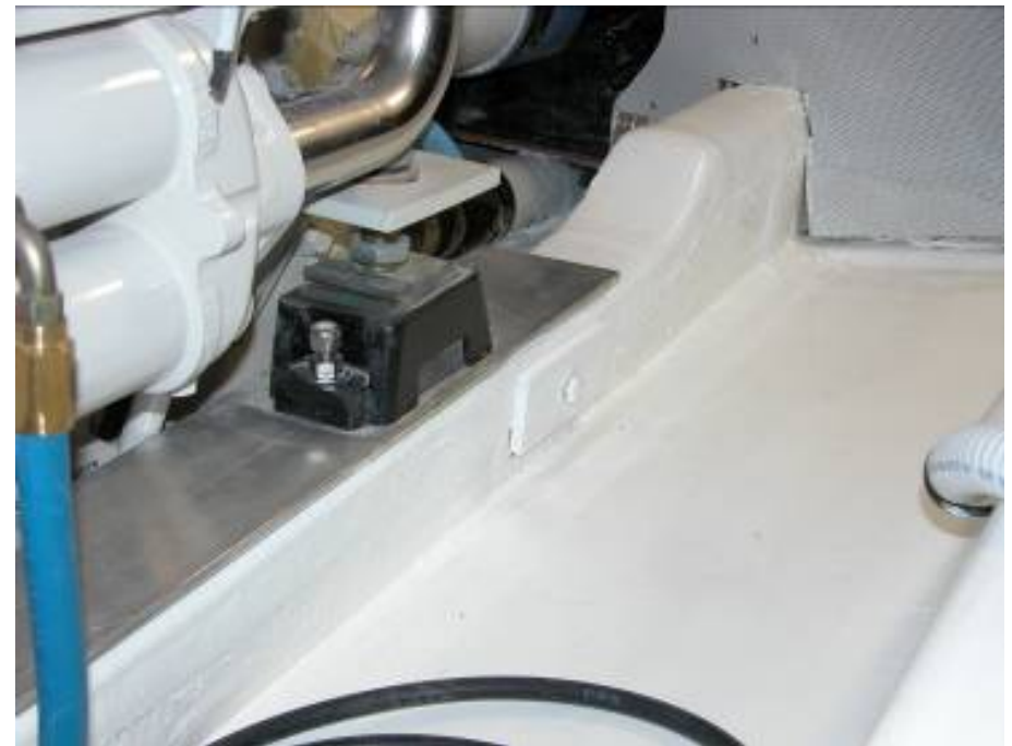
Aluminum saddle is fitted to composite girder
