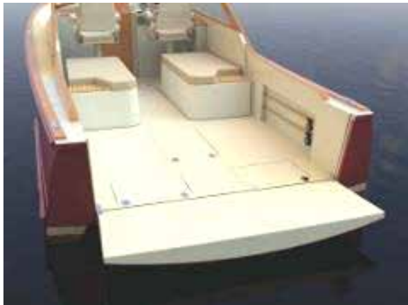
Hinged Transom featured on 10 m Yacht from C.H. Marine Yachts, Shelter Island, NY
