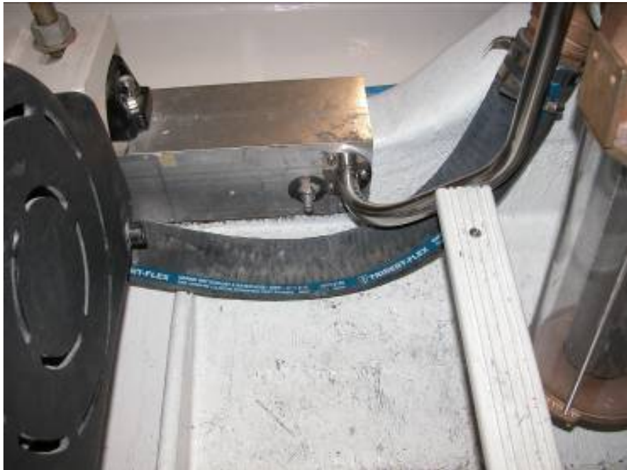
Aluminum saddle is fitted to composite girder
