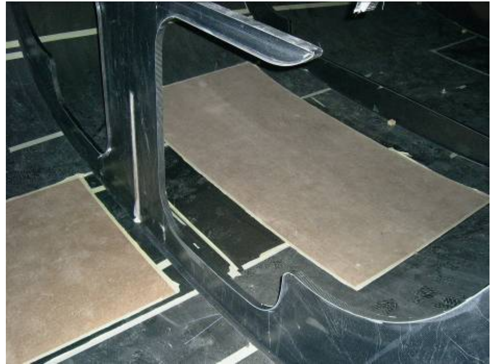
This carbon fiber/Nomex bulkhead has the attachment flange molded with the bulkhead and bonded to the hull with a flexible epoxy adhesive
