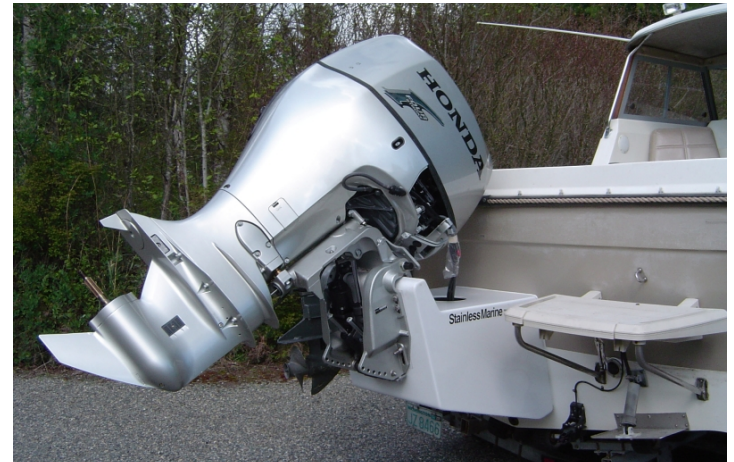
Contemporary outboard bracket with internal bracket support
