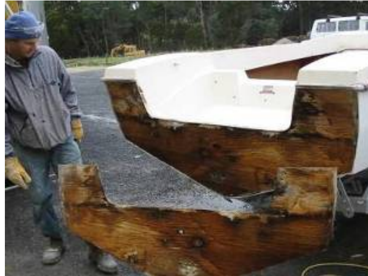
A water-saturated transom undergoing repair at Penguin Composites in Australia
