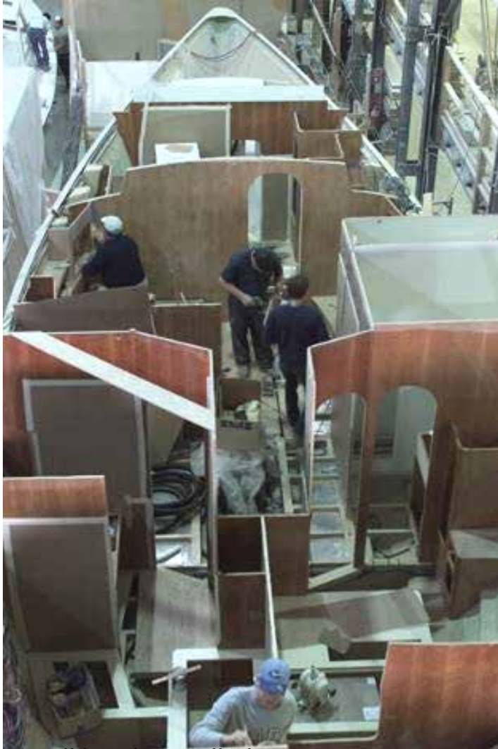
Bulkheads installed in epoxy composite 54' sloop from Alden Yachts of Portsmouth, RI
