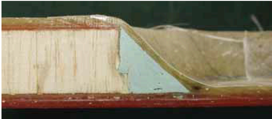
Example of through-hull close-out showing putty used to create fillet
