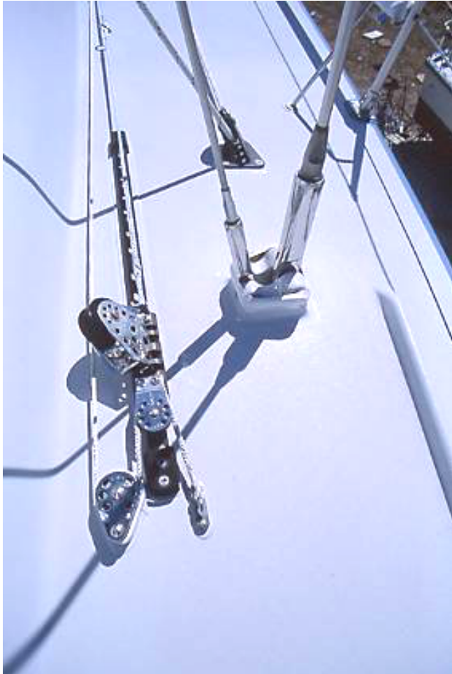
Composite chainplates featured on 15 meter IMS racer built by New England Boatworks
