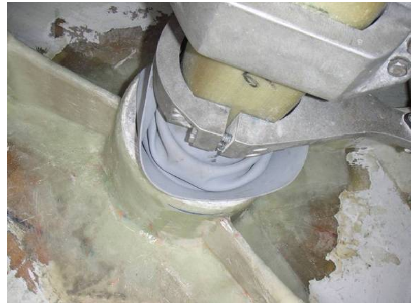
Recommended Jefa bearing installation detail for tiller steering
