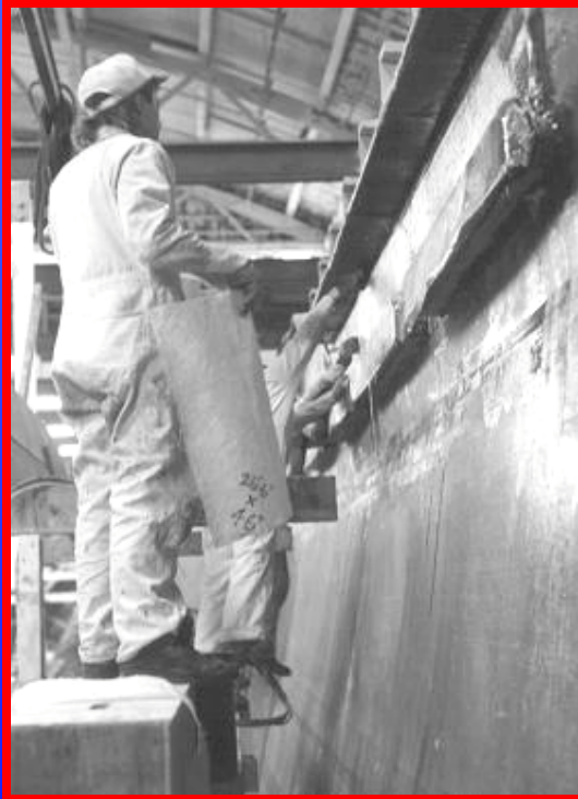
Workers Laminate Side of Large Hull
