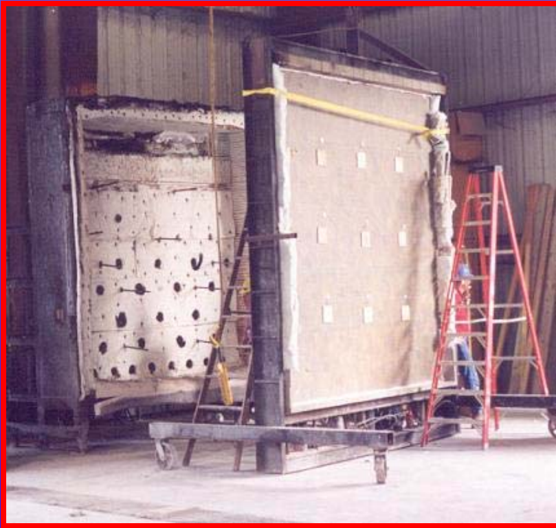
Test Arrangement for Burn Through Resistance of 10 x 10 - foot Panel
