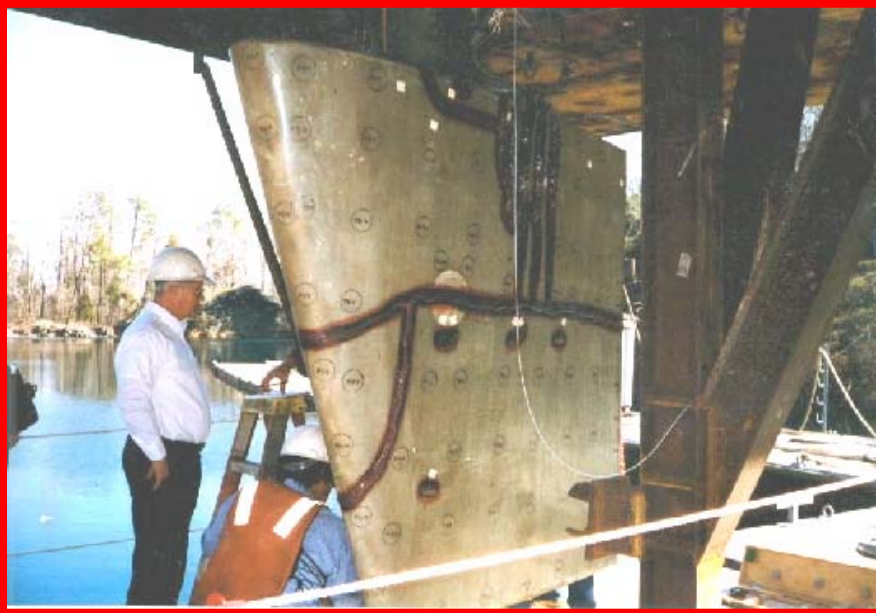
Composite MCM Rudder Built by Structural Composites Shown During Shock Trials
