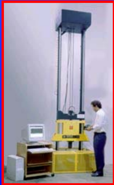
Instron's Dynatup® 8100 Series Drop Weight Impact Test System Can Handle Impact Energies up to 20,500 ft-lbs and Impact Velocities up to 22 ft/s
