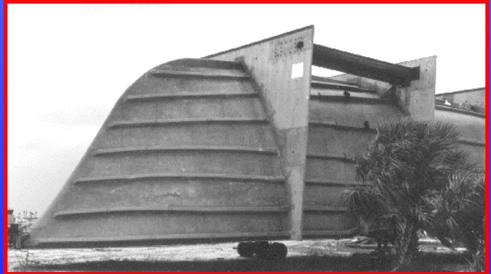
Large Female Mold with Stiffeners
