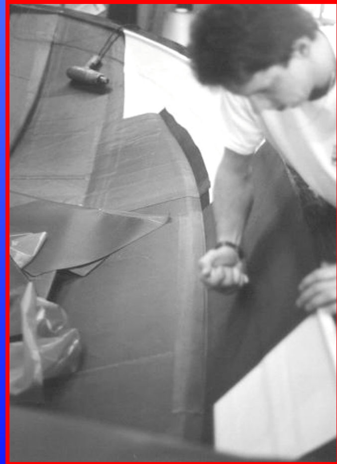
Prepreg Material Consolidated Prior to Cure
