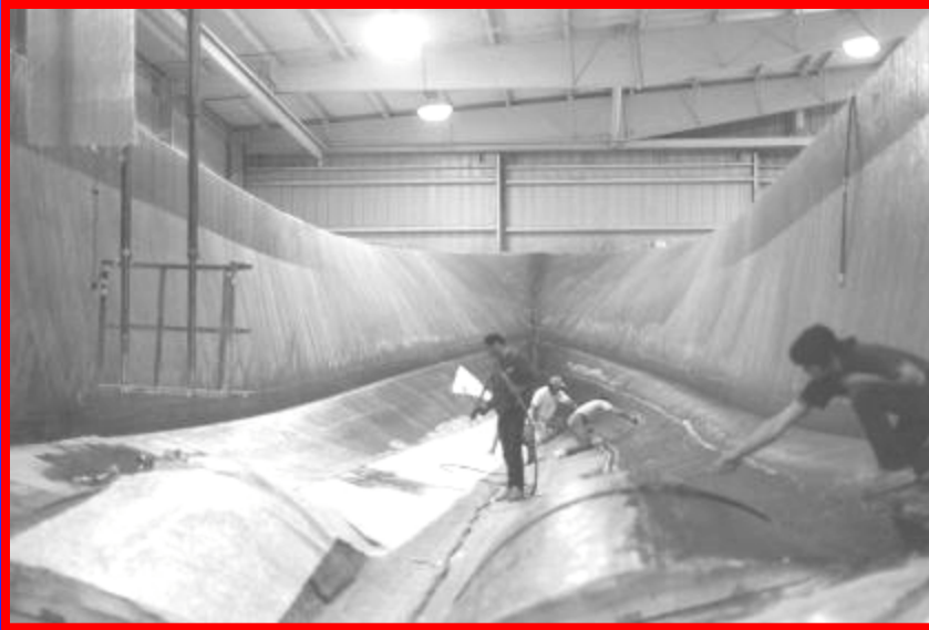
Hand Layup of Solid Laminate Hull at Westport Marine
