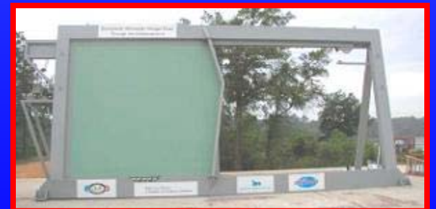
Composite Helicopter Hanger First Article Door (above) and Operational Test Jig (below) [Seemann Composites]
