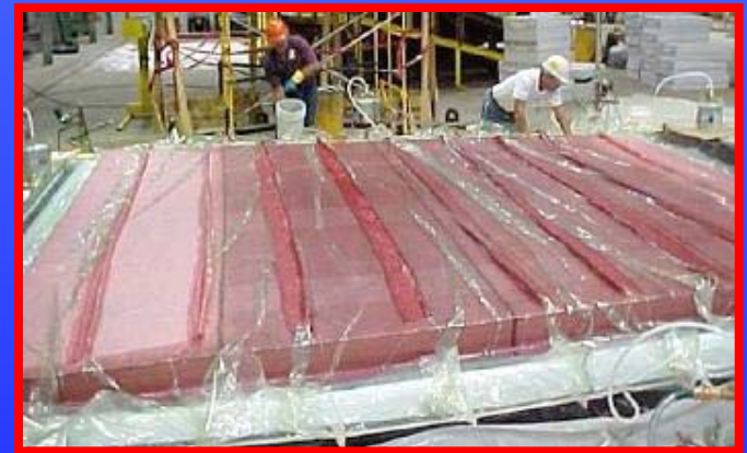
Sandwich Panel Being Fabricated by Northrop Grumman Ship Systems Using the SCRIMP Method
