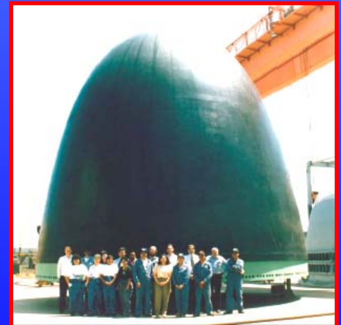
Composite Submarine Bow Dome Produced by Goodrich Composites
