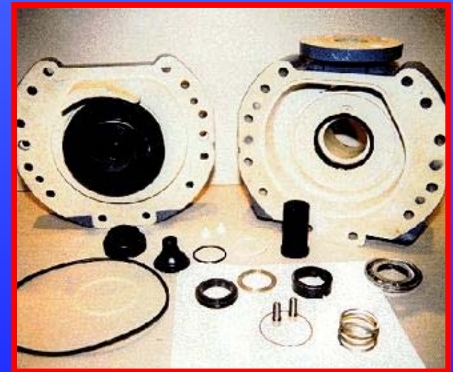
Navy Shock-Qualified Composite Pump Internals Built by Flowserve
