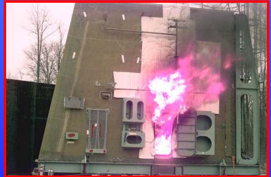
Full-Scale Fire Test for Helicopter Hanger Project with Fire Protection Around Door for Fire Test Only
