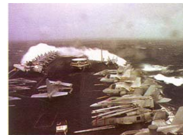
Saltwater Spray Environment on Aircraft Carrier [OSD Corrosion Control]
