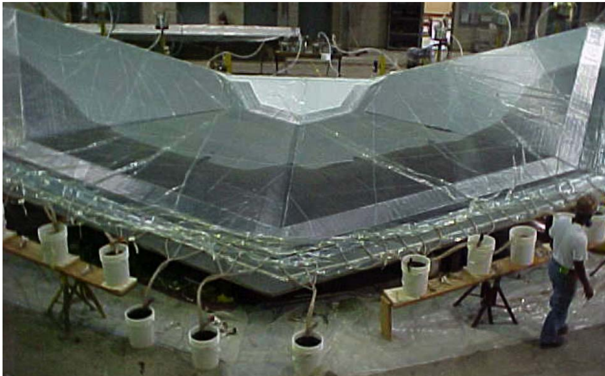
Infusion of AEM/S Panel at NGSS [Rasmussen, NSWCCD]
