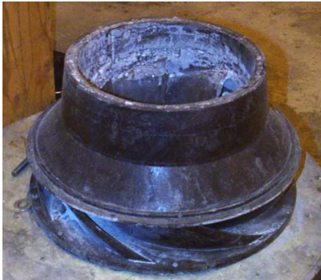
Composite Marine Impeller [Piet Van Dine, GD Electric Boat]
