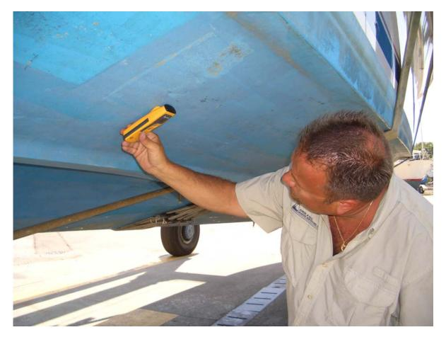
Figure 2. A Marine Surveyor Uses a Moisture Meter to Examine a Boat Bottom [http://www.powerandsailmarinesurveyors.com/serv01.htm]
