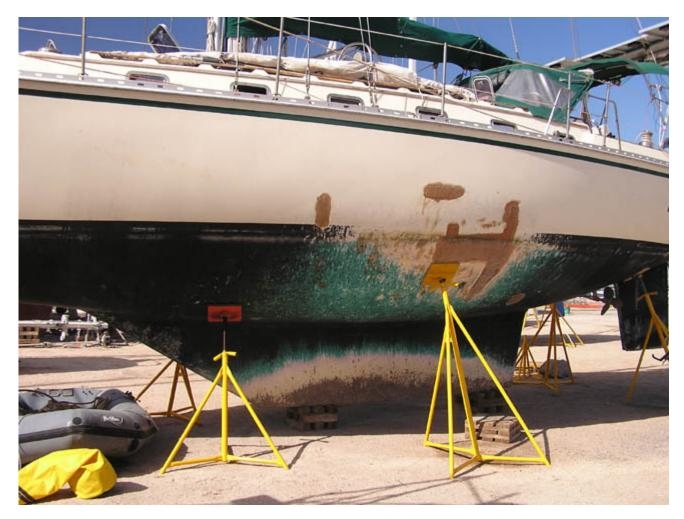
Figure 1. Visual Inspection of Hull Damage from Grounding Showing Temporary Repair [http://svmirador.net/February\_8\_2004.htm]
