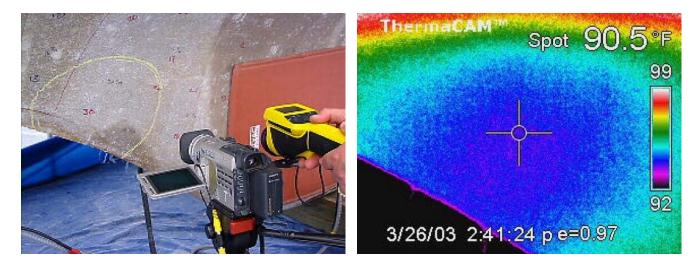
Figure 3. Water Intrusion Documented with Infrared Camera [http://allinson.com]
