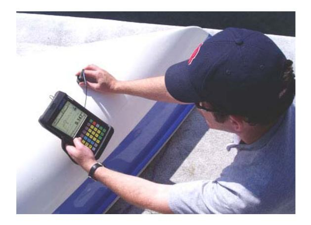
Figure 4. Ultrasonic Thickness Measurement Gage Used to Determine Thickness of a Sailboat Racing Hull [http://www.olympusndt.com/en/ndt-application/87-id.209715260.html]
