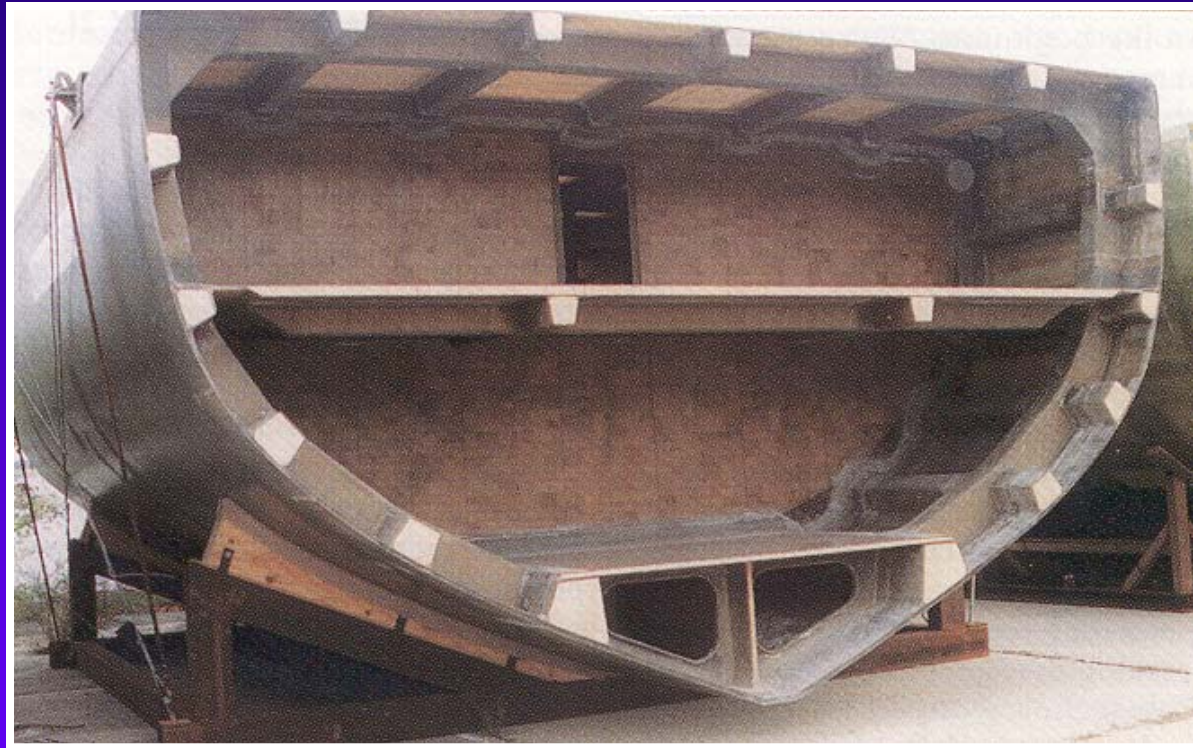
Midship Section of 1/2 Scale Corvette Built by Seemann Composites for NSWCCD
