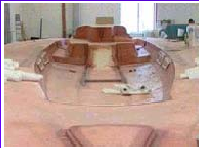
Deck Being Molded at Sabre Yachts
