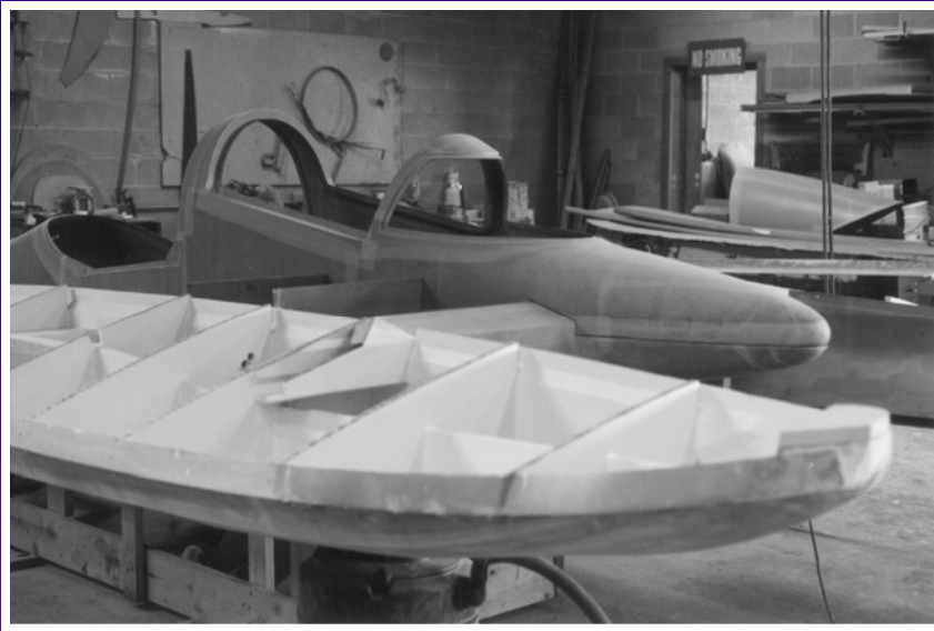
Prepreg/Nomex Honeycomb Core Construction of Hydroplane at Ron Jones Marine
