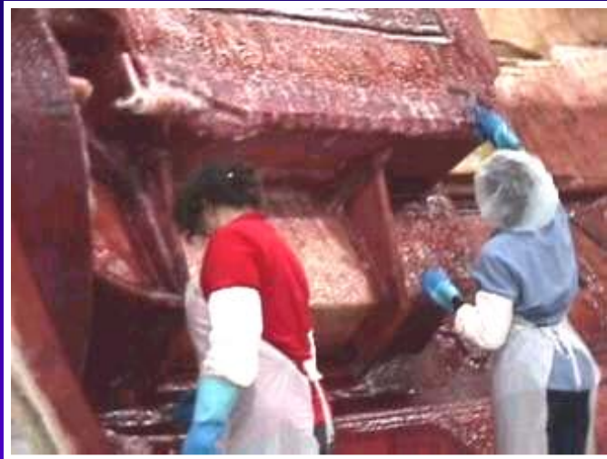
Deck Layup at Beneteau USA
