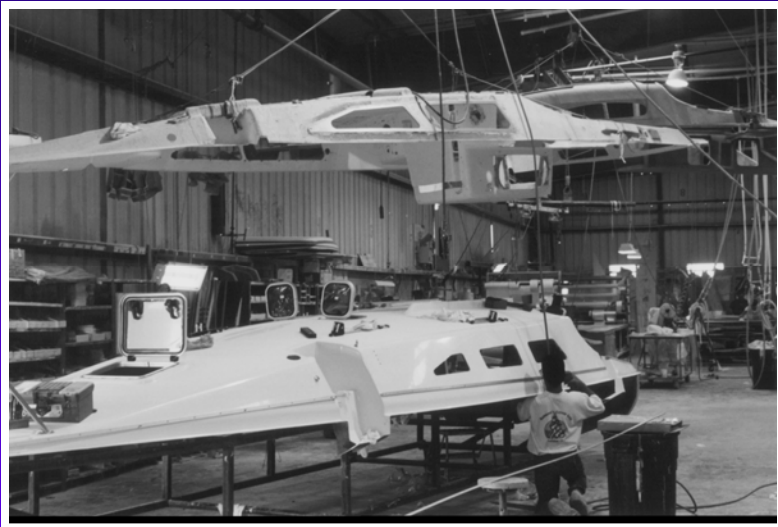
Hardware Placement Jig Lowered in Place at Corsair Marine
