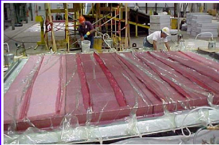
Panel Being SCRIMPed at Avondale Gulfport Facility
