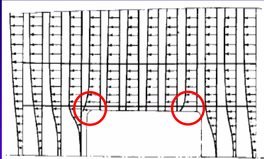
Distribution of Longitudinal Stress at Hatch Opening from C.S. Smith
