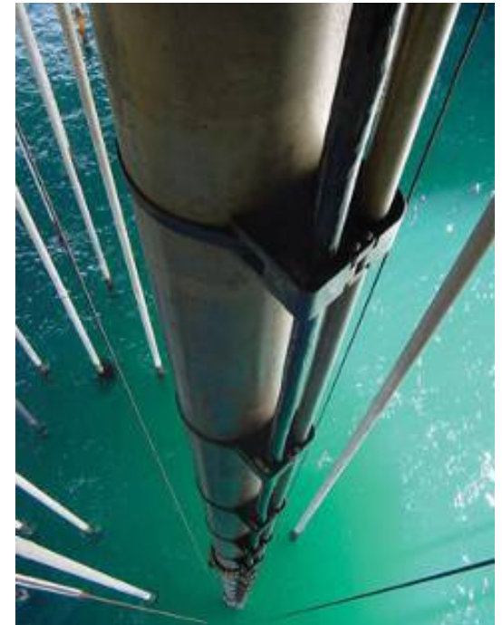
Composite Drilling Riser Developed by Aker Kvaerner Subsea
