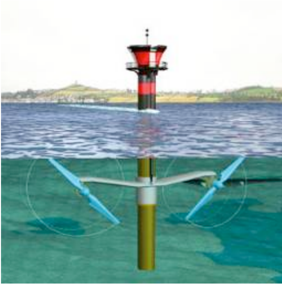
Marine Current Turbines Ltd has installed a 1.2MW SeaGen tidal energy system in Ireland.
