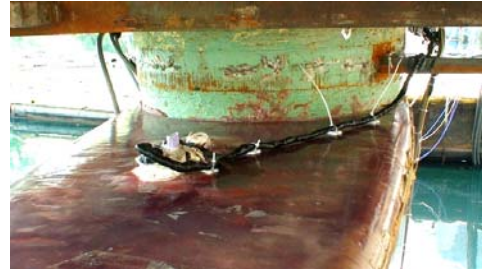
Figure 23. Strain Gauge Cabling for DDG 51 Rudder Shock Tests
