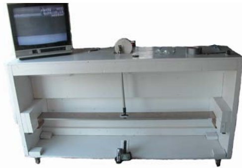
Figure 29. Panel Coating Fatigue Test Apparatus Developed for SSC-442 [ref 38]
