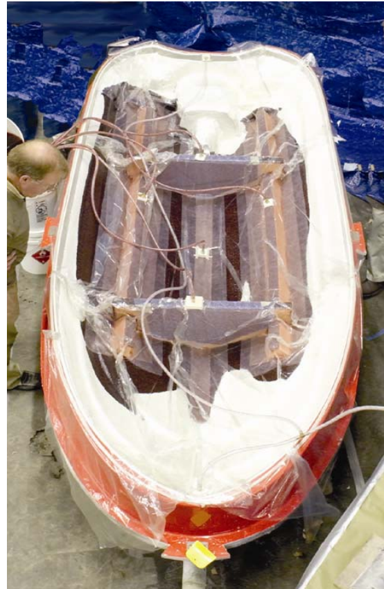
Figure 4. Boat hull infusion (courtesy of Colbond)
