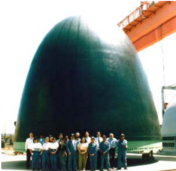
Composite Submarine Bow Dome Infused with Epoxy by Goodrich Composites
