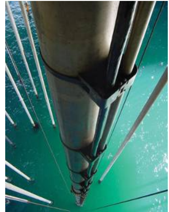
Composite Drilling Riser Developed by Aker Kvaerner Subsea
