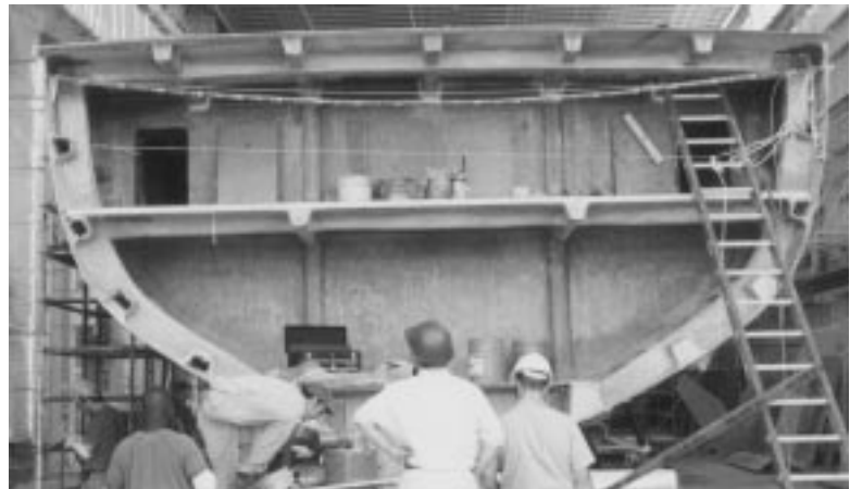
Figure 5-49 One-Half Scale Corvette Hull Test Section Built for the U.S. Navy Using the Sunrez ™ Process [author photo]
