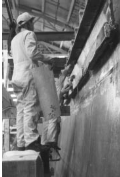
Figure 5-18 Workers Laminate Hull at Northcoast Yachts [author photo]
