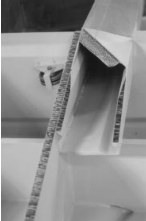
Figure 5-42 Deck Beam Showing Honeycomb Core Construction at Ron Jones Marine [author photo]
