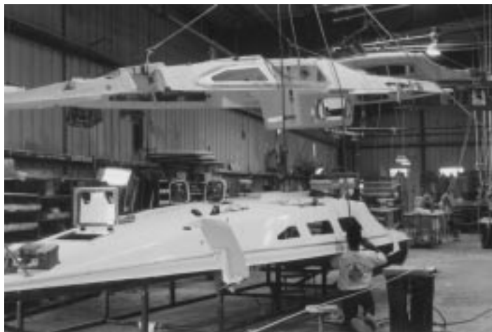
Figure 5-20 Hardware Placement Jig is Lowered Over Recently Laminated Deck at Corsair Marine [author photo]
