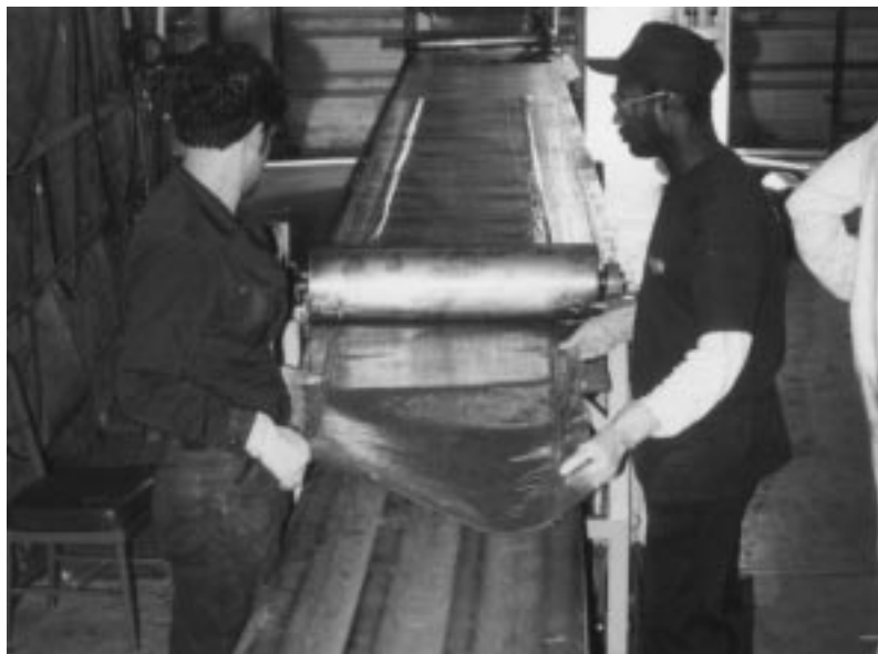
Figure 5-46 Prepreg “Bundle” of Six Layers of Unidirectional E-Glass is Passed Through Consolidator for a Stiffener by Composite Ships [author photo]
