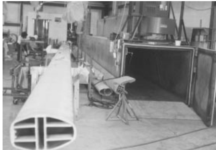
Figure 5-44 Cure Oven Used for Masts and Hardware at Goetz Marine Technology [author photo]
