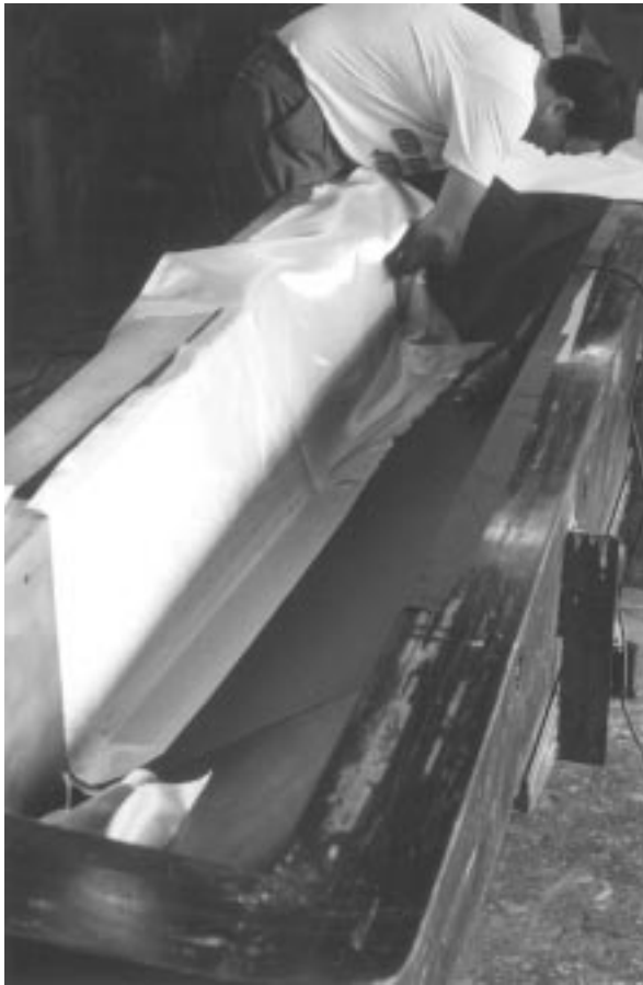
Figure 5-40 Prepreg Material is Positioned in Mold at Ron Jones Marine [author photo]
