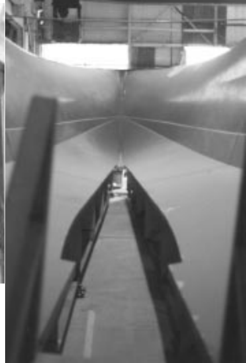
Figure 5-7 Expandable Female Mold at Northcoast Yachts [author photo]
