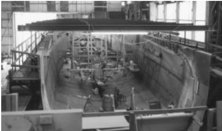
Figure 5-16 Hull and Scaffolding Set Up at Northcoast Yachts [author photo]
