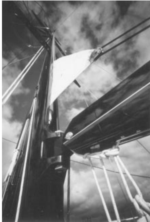
Figure 1-9 150-foot Omohundro carbon Fiber/Epoxy Mast for 115' Ted Hood Designed Shallow Draft Sailing Yacht Built by Trident Shipworks [photo by the author]
