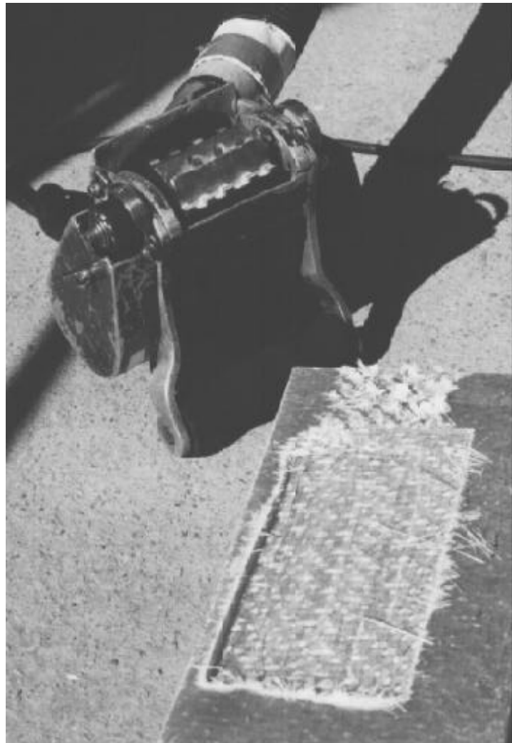
Figure 5-53 Laminate Peeler Developed by Osmotech with a Thick-Sectioned Laminate After One Pass [author photo]
