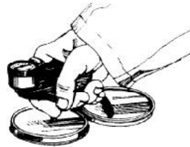
Figure 5-71 Barcol Impressor (Model 934 or 935 for readings over 75) [Cook, Polycor Polyester Gel Coats and Resins ]
