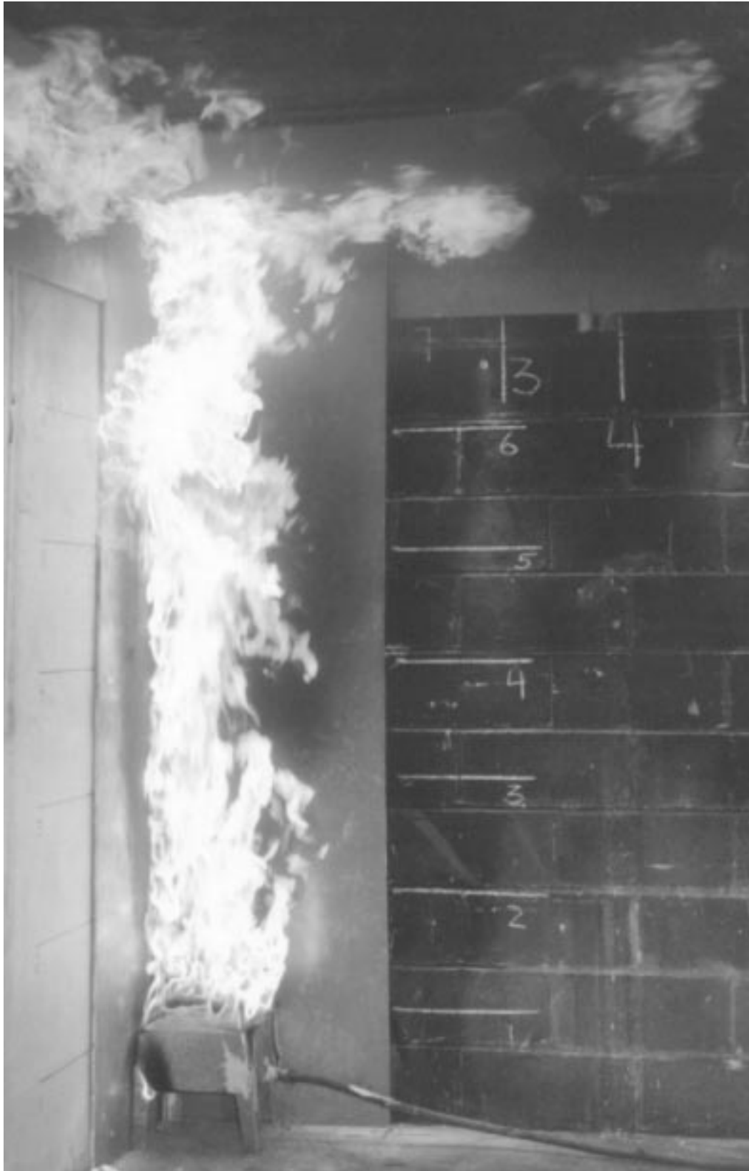
Figure 4-47 ISO 9705-Type Test with Reduced Material Quantities at VTEC Laboratories Showing 300 kW Burner Output [author photo]
