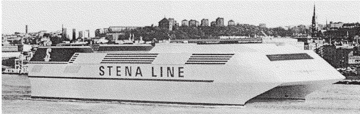
Figure 1-12 Finnyard's Stena HSS (High Speed Sea Service) 124 Meter Ferry Features the Use of Composites for Bulbous Bow Sections, as well as for Stacks, Stairwells, A/C Spaces and Interior Furniture [Fast Ferry International]
