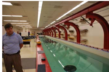
Figure 29. Above is A Schematic of the U.S. Naval Academy's 120-foot Wave Tank. At Right is Co-Investigator Mark Krawczewicz alongside the Tank. Below are Photos of the Tank's Wave-making Mechanism
