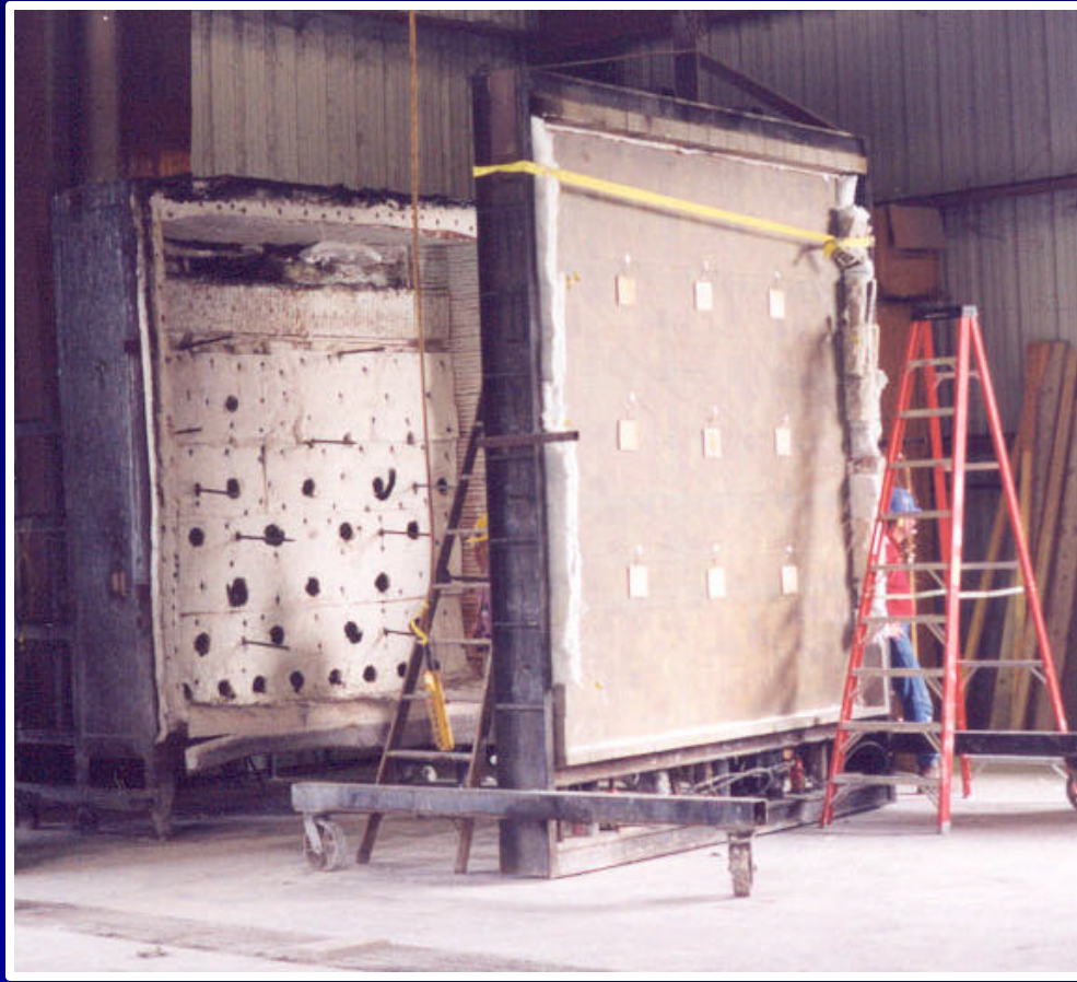
Test Arrangement for Burn Through Resistance of 10 x 10 - foot Panel
