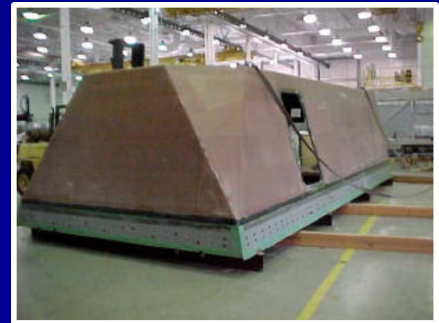
Composite Helicopter Hanger for DDG 51 Flight IIA Destroyer Built at Northrop Grumman Gulfport Facility
