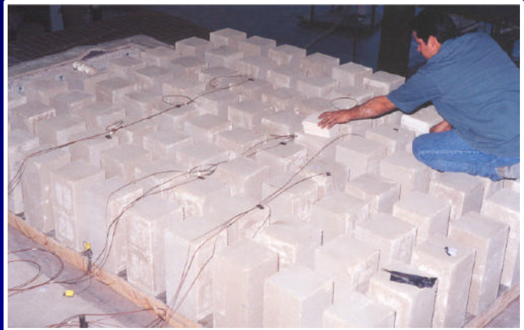
Weights Being Positioned for Deck Test at Omega Point Laboratories
