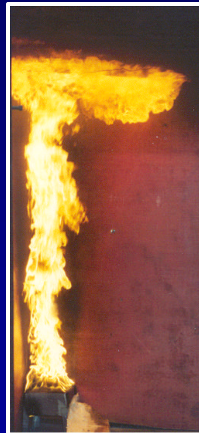
Flame Spread Testing with ISO 9705 Room Corner test
