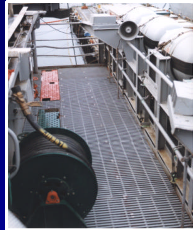
Phenolic Deck Grating Installed on Aircraft Carrier
