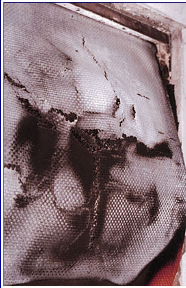
E-Glass Vinyl Ester Laminate Tested Without Insulation for Burn Through Resistance
