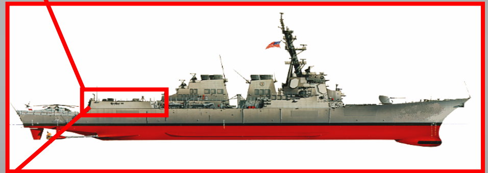
Composite Helicopter Hanger for DDG 51 Flight IIA Destroyer Built at Northrop Grumman Gulfport Facility
