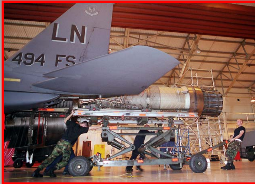
Strike Eagle jet engine change Crew Chiefs from the 48th Fighter Wing, United Kingdom, pull out a Pratt & Whitney F100-229 engine from a F-15E Strike Eagle
