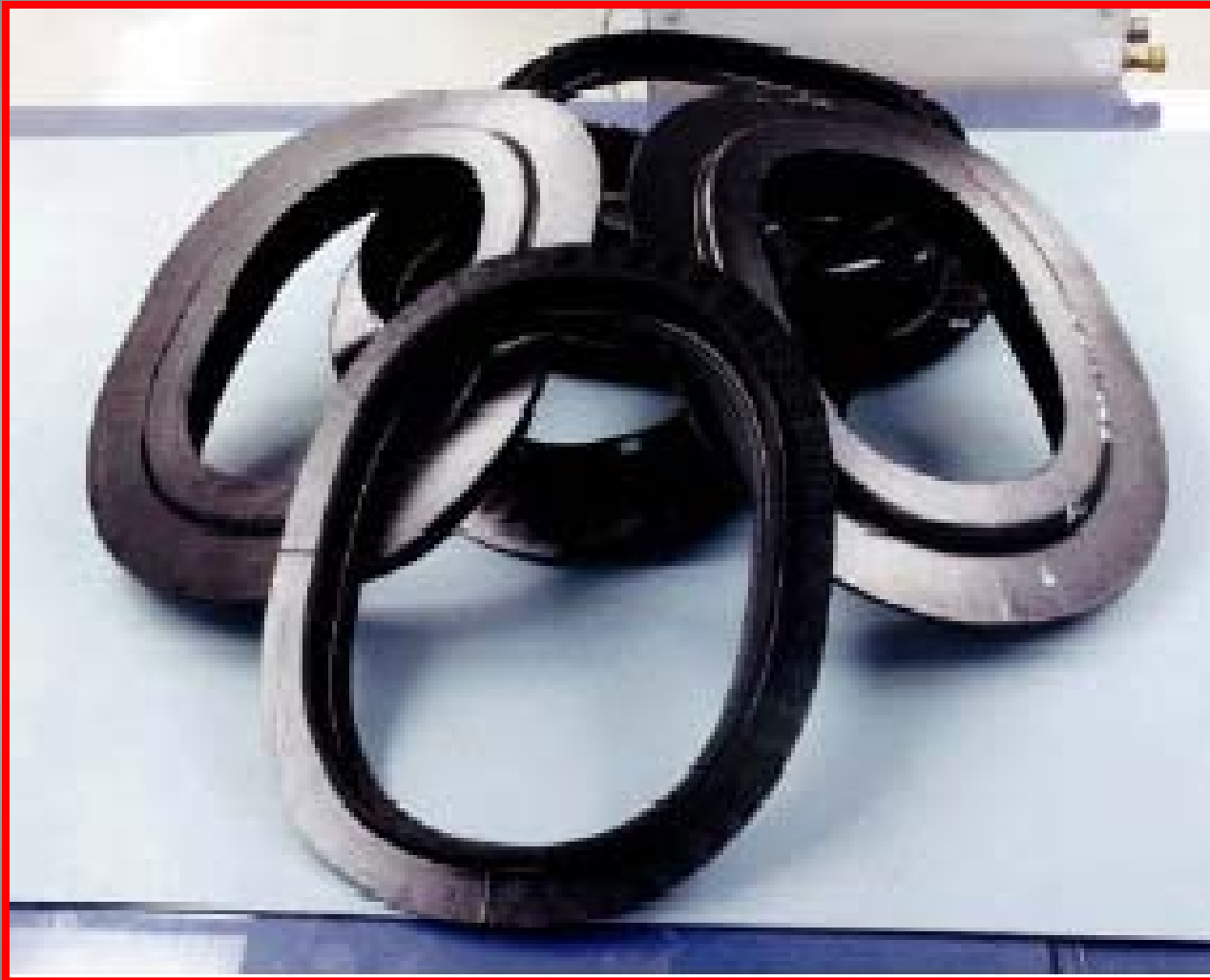
Completed Braided and Woven Window Frames
