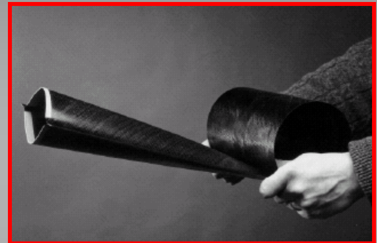
Epoxy/Carbon Fiber Deployable Boom
