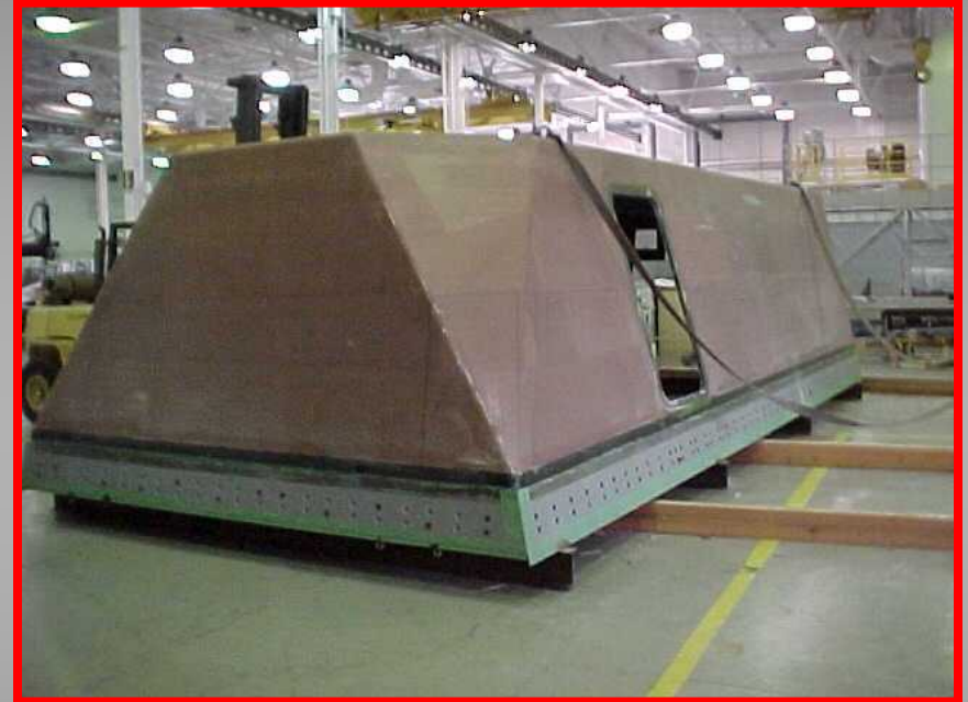
Forward Director Room Built by Northrop Grumman as Technology Demonstrator for DDG 51
