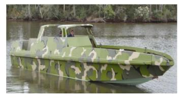
The 42-foot Advanced Composite Riverine Craft was developed by Seemann Composites based on resin infusion
