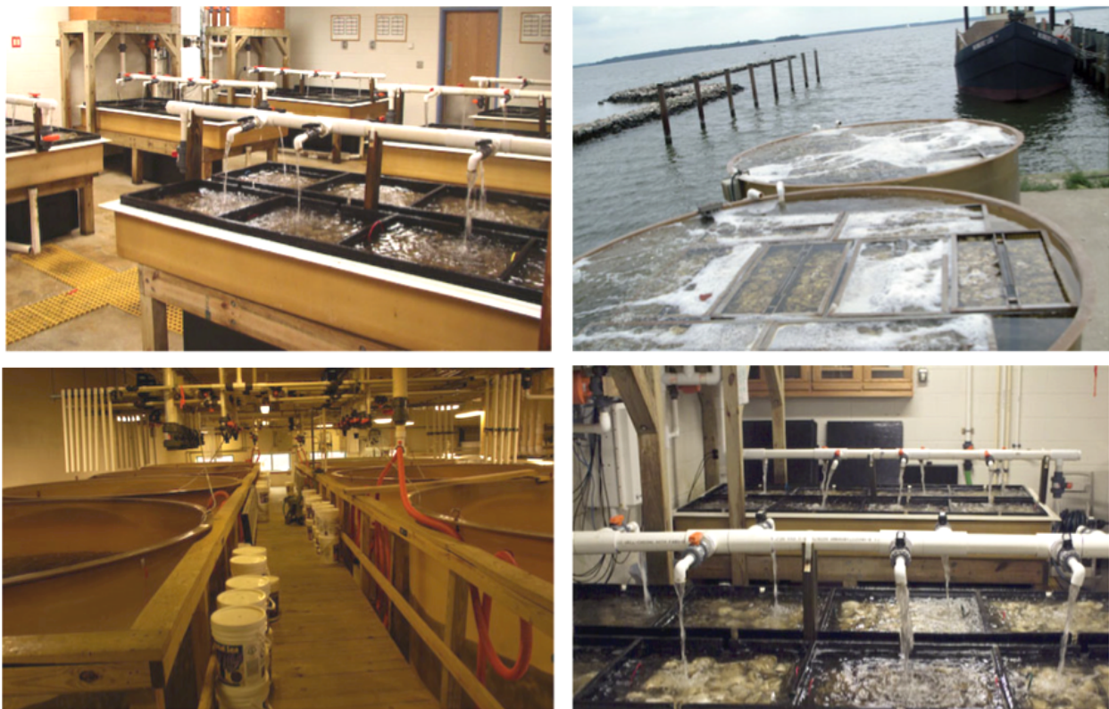
Figure 20. Broadstock conditioning tables (upper left); setting tanks (upper right); mass larval tanks (lower left) and conditioning system (lower right) at the 6000 m 2 Aquaculture and Restoration Ecology Laboratory at the Horn Point Laboratory [ http://www.umces.edu/hpl ]
