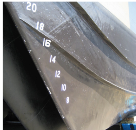
Figure 16. Silicon antifouling treatment on Norwegian surface effect ship [author photo]
