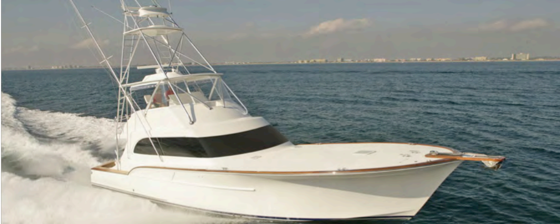
Figure 9. The bow flare on this 58' sportfisherman from Davis Boats is typical of this genre http://www.davisyachts.com/wp-content/uploads/2014/10/Davis-58SF-Run_HOME_2.4.jpg
