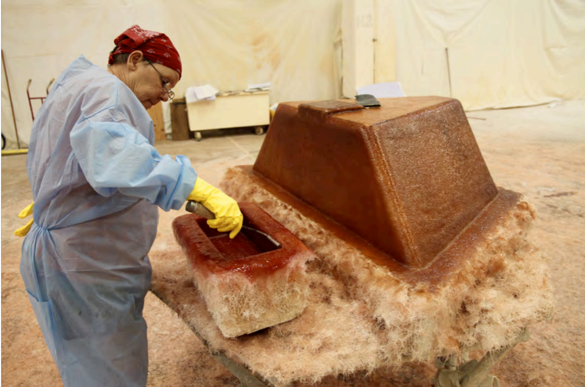
Figure 17. Hand layup remains an economical method for manufacturing smaller boats and parts http://parkerboats.net/wp-content/uploads/2013/08/19-Laminating-Small-Parts.jpg
