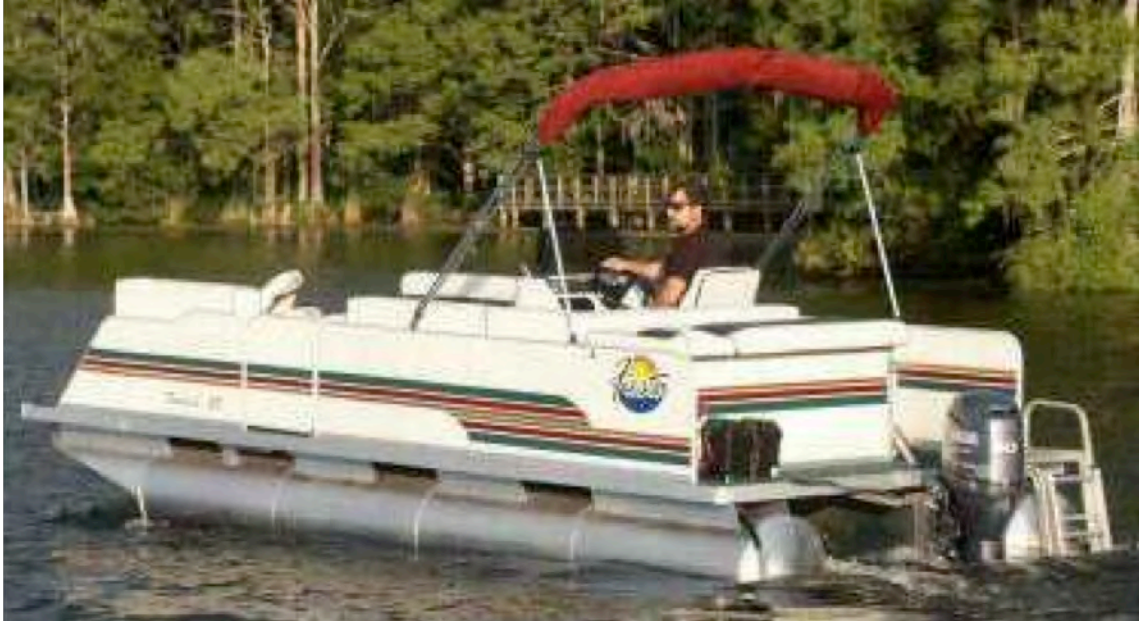
Figure 11. Pontoon boats are designed to be built using aluminum structural profiles http://www.travelizmo.com/archives/fiesta-fundeck-pontoon-boat-2008.jpg
