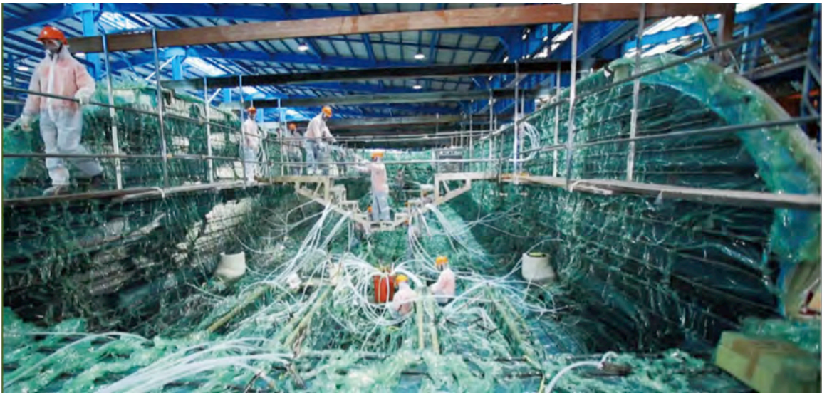
Figure 18. This complex labyrinth of vacuum and resin supply lines is typical for infusing a large hull https://www.horizonpowercatamarans.com/wp-content/uploads/2014/10/Screen-Shot-2014-10-21-at-2.08.44-PM.png
