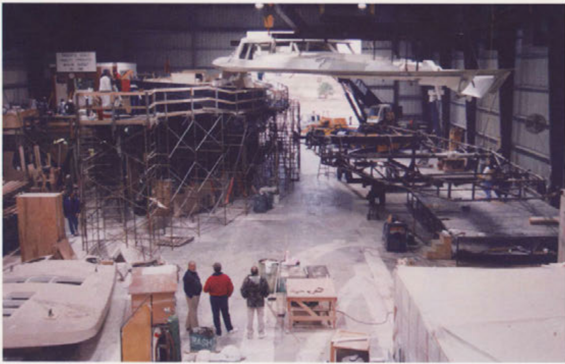
TEEL's deck is lifted for final placement after several dry runs where flanges were built to guarantee a close fit. TEEL's hard top is seen off to the left.
