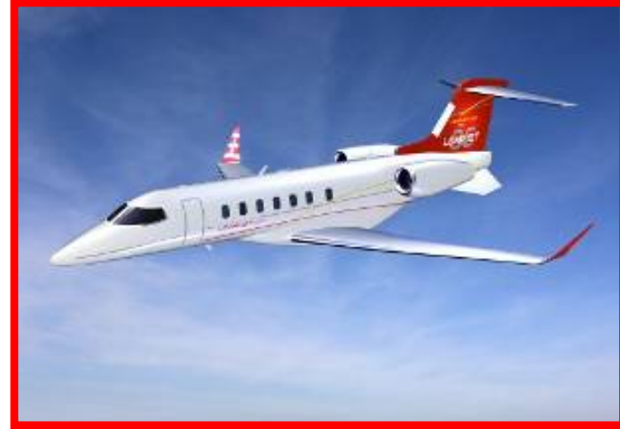
Bombardier Aerospace new mid-size business jet is an all-composite design
