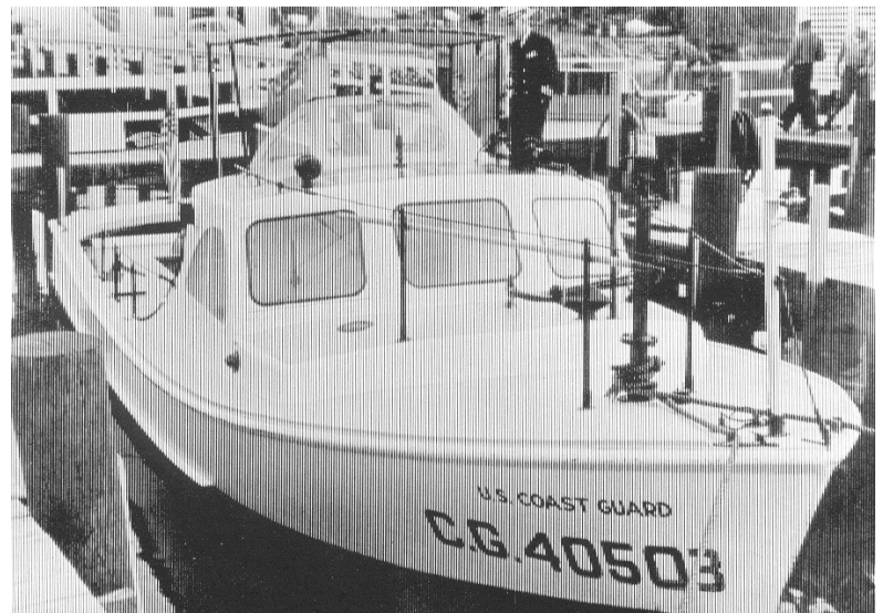
Figure 3. USCG Hull 40503 [Owens-Corning Fiberglass, Fiber Glass Marine Laminates, 20 Years of Proven Durability]
