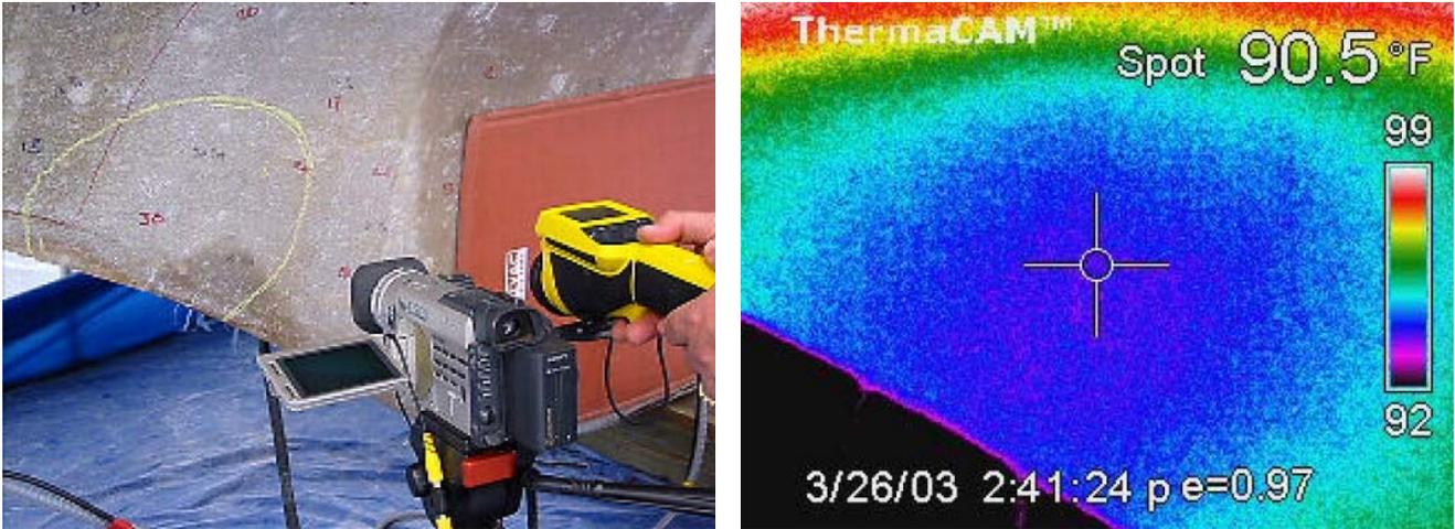
**Figure 3. Water Intrusion Documented with Infrared Camera [<http://allinson.com>]**
