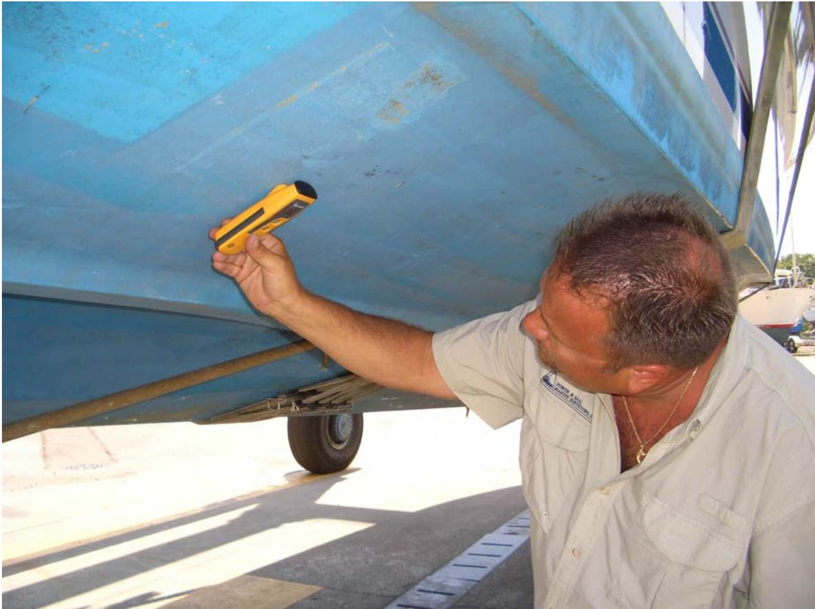
**Figure 2. A Marine Surveyor Uses a Moisture Meter to Examine a Boat Bottom**
