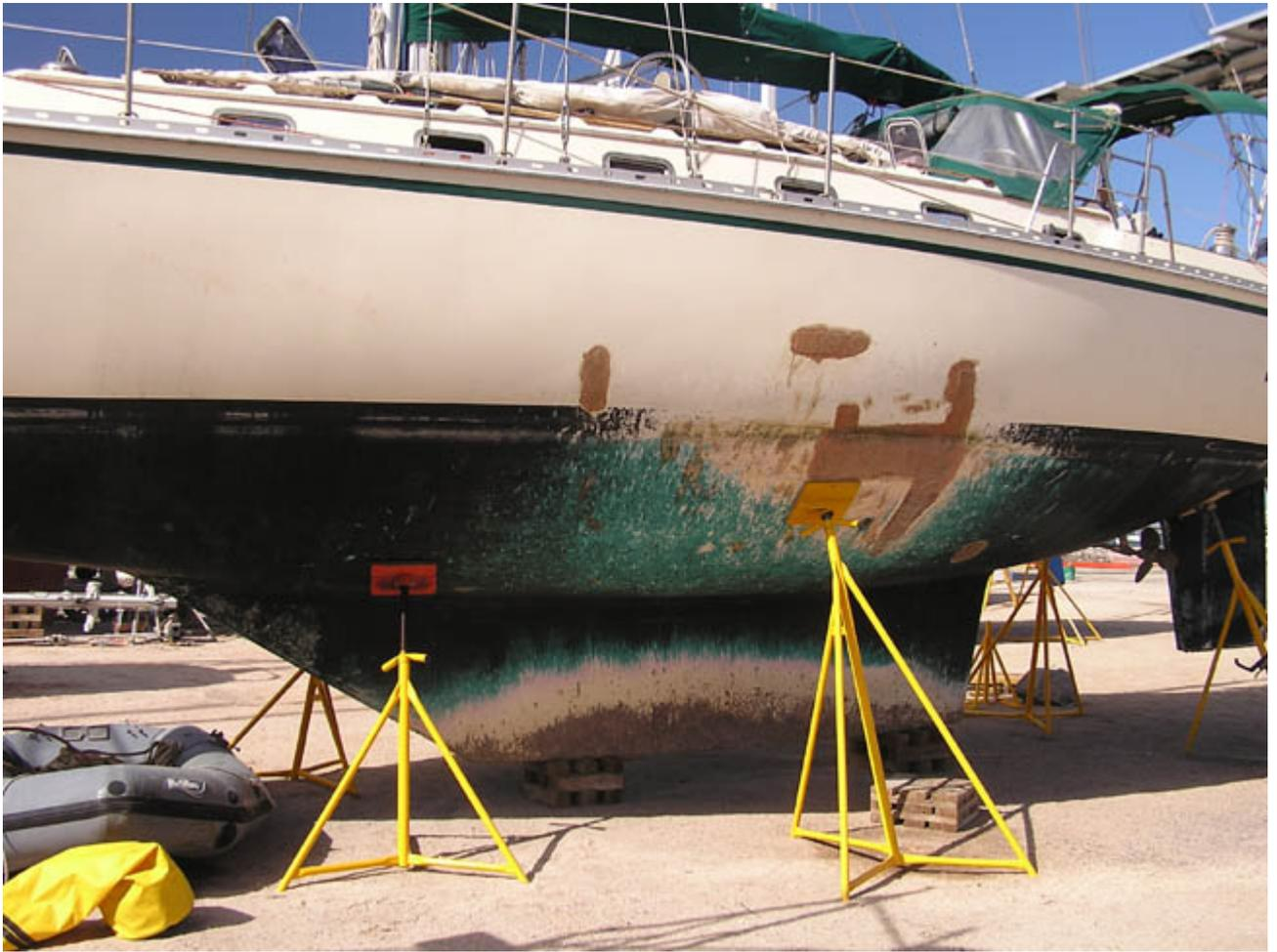
**Figure 1. Visual Inspection of Hull Damage from Grounding Showing Temporary Repair [[http://svmirador.net/February\\_8\\_2004.htm](http://svmirador.net/February_8_2004.htm)]**
