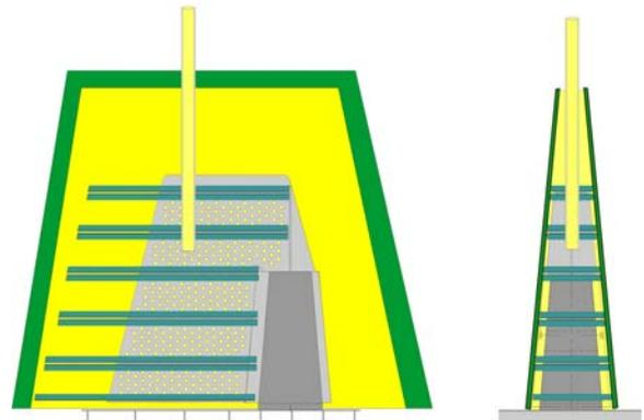
Wrap Steel/Foam Structure with Dry Reinforcement with Hub Supported on Pedestal
