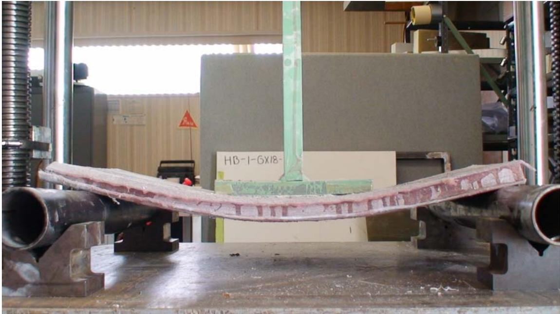
**Figure 3. Structural Testing of Steel/Composite Interface Joint**
