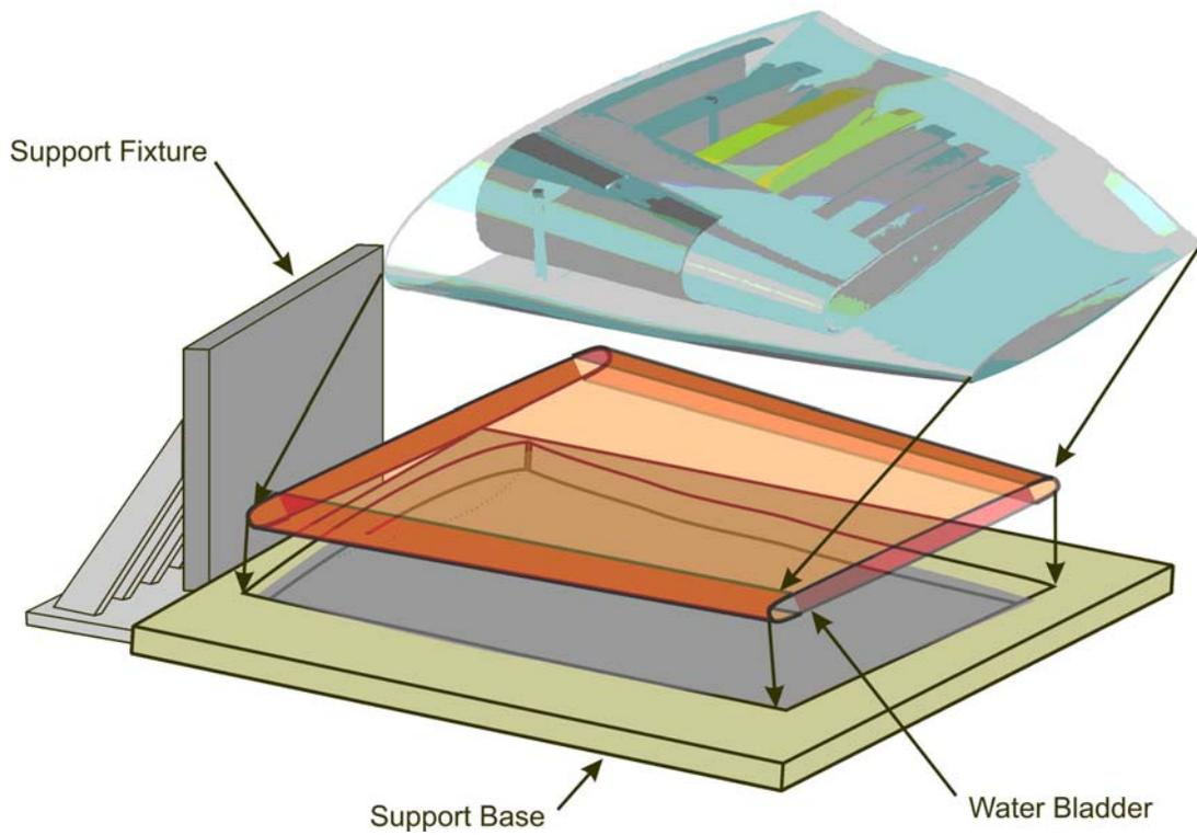
**Figure 4. Plan for Full-Scale Static Testing**
