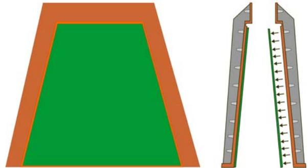
First Injection of Foam Using Mold
