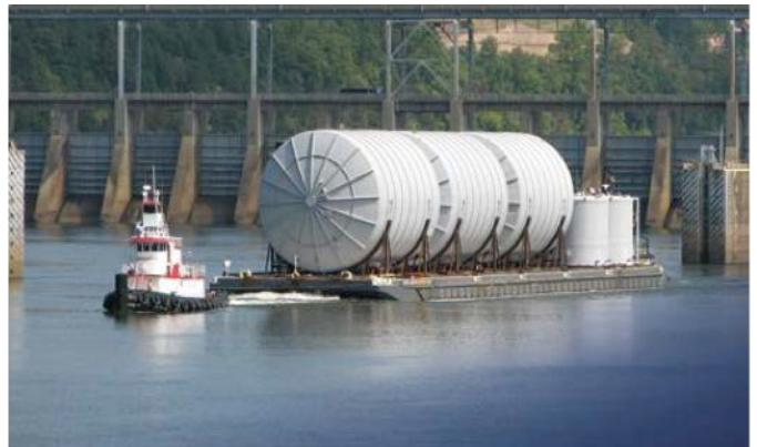
These very large storage tanks were fabricated from glass fiber-reinforced plastic by Ershigs Inc. to contain hydrochloric acid.
