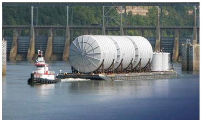
These very large storage tanks were fabricated from glass fiber-reinforced plastic by Ershigs Inc. to contain hydrochloric acid.
