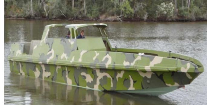
The 42-foot Advanced Composite Riverine Craft was developed by Seemann Composites based on resin infusion
