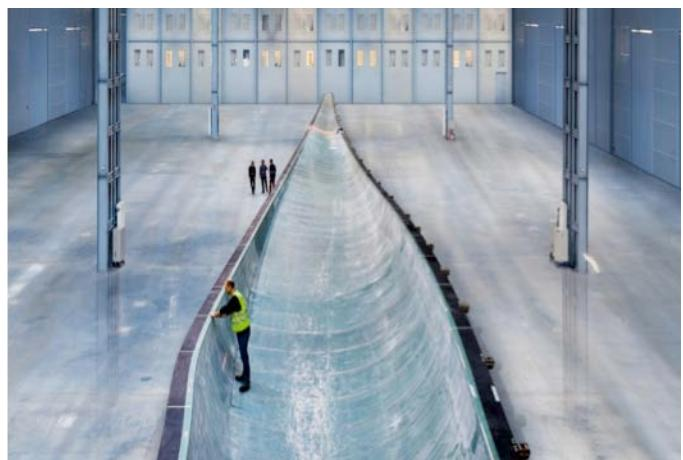
This 75 meter wind turbine blade built by Siemens consists of a single component made from epoxy resin and balsa reinforced with glass fiber.
