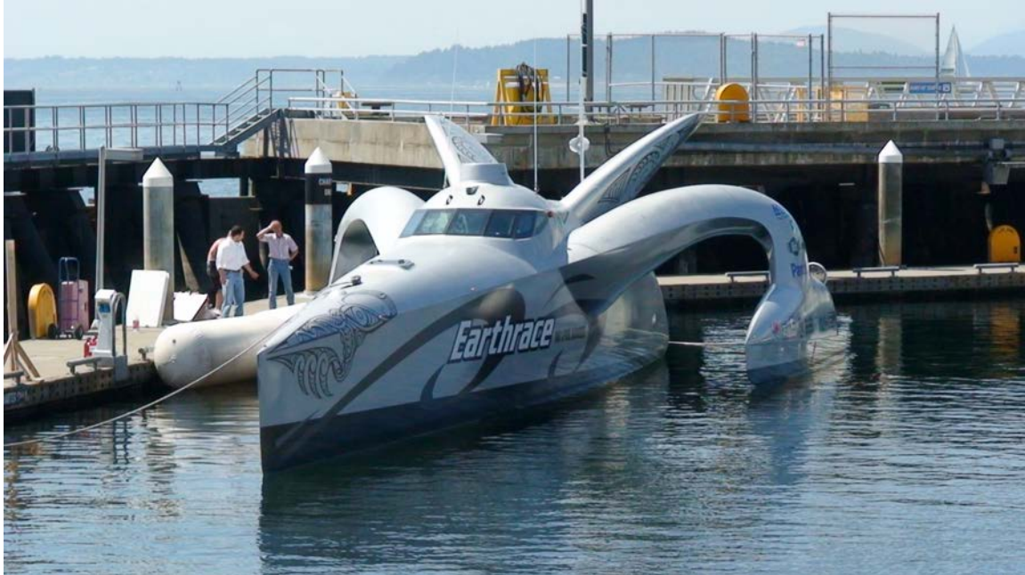
Figure 4. Earthrace holds the record for a powerboat to circumnavigate the globe at just under 61 days. The boat was run on 100% biofuel, claiming a net carbon zero footprint in order to draw attention to the need for renewable fuels and sustainable living. Earthrace was built in Auckland, New Zealand, by Calibre Boats, who specialize in high-tech composite boatbuilding. The hull is made from sandwich composites using 40mm of PVC foam core sandwiched between three layers of carbon inside and out, with a layer of Kevlar ® for impact resistance on the outside (albeit, insufficient to resist being rammed by a Japanese whaling vessel during a confrontation in 2010).
