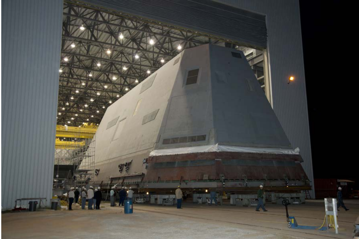
Figure 3. At about 900 tons (outfitted), the DDG 1000 destroyer deckhouse is claimed to be the largest composite structure ever built. To reduce radar cross-section, ship antennas (apertures) are embedded directly in the structure itself. Huntington Ingalls Industries claims they can build panels up to 150 by 50 feet and assemble large structures to a tolerance of less than 1/8th of an inch.
