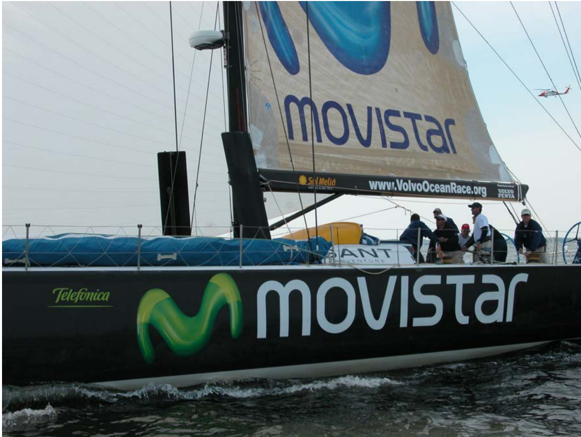
Figure 5. movistar was built to the Volvo Open 70 rule for the 2005-6 Volvo Ocean race. She is pictured here sailing down the Chesapeake Bay on way to New York. The boat sank on the next leg of the trip to Portsmouth, UK after her aft keel bearing collapsed and broke away from the hull allowing water to pour into the hull. The boat was built by the Australian yard Boatspeed using 70°C cure prepregs and Corecell™ foam core from SP Systems (now Gurit).
