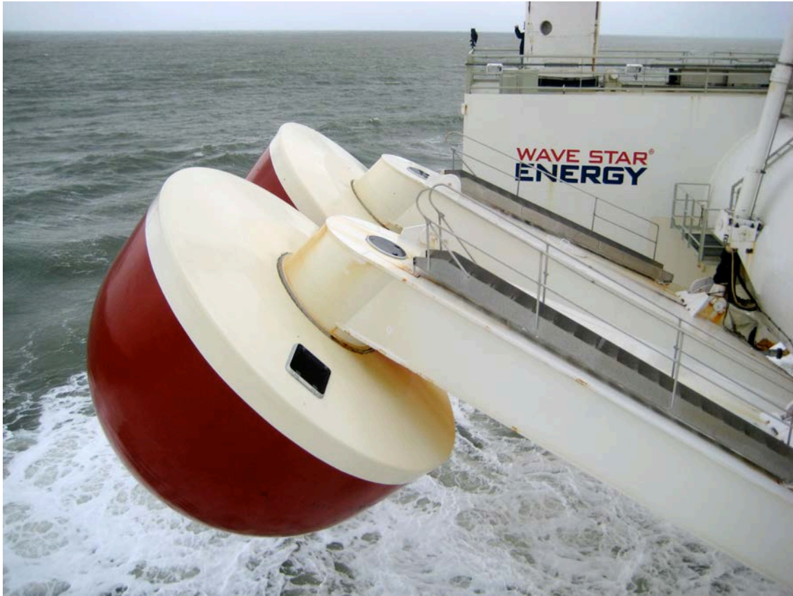
Figure 10. The Wave Star ® Energy marine hydrokinetic energy concept was invented by sailing enthusiasts Niels and Keld Hansen in 2000. The half-submerged buoys rise and fall, allowing energy to be continually produced despite waves being periodic. The buoyancy of the float is 20-40 times its dry weight, made possible by composite construction.
