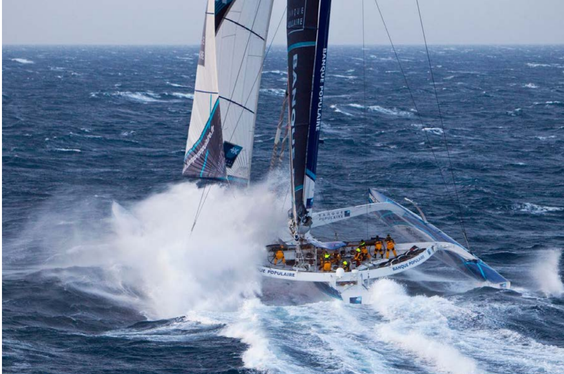
Figure 2. Three and a half years after being launched in August 2008 and after her second attempt, the Maxi Banque Populaire V has won the Jules Verne Trophy with a circumnavigation that took just over 45 ½ days. Loïck Peyron and his crew covered 29,002 miles at an average speed of 26.51 knots. The 40-meter trimaran was built by CDK Technologies in the Brest region of France using advance composite materials.
