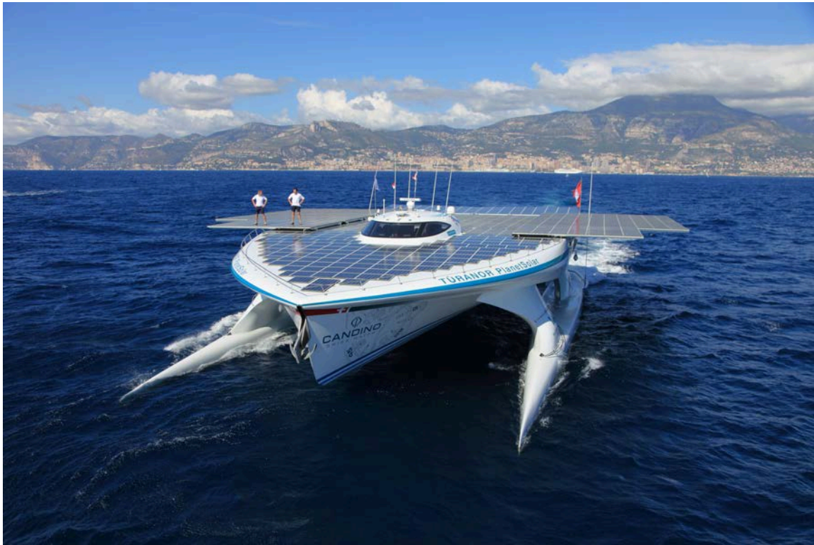
Figure 6. The Turanor PlanetSolar , is a 31meter wavepiercer catamaran with approximately 537 square meters of solar panels on its deck that drive highly efficient carbon fiber propellers. Designer Craig Loomes from New Zealand specified advanced carbon fiber hull construction to achieve a 65,000 kg displacement. The boat was completed by the Kiel, Germany yard of Knierim Yachtbau in 2010 and completed a circumnavigation voyage in May 2012.
