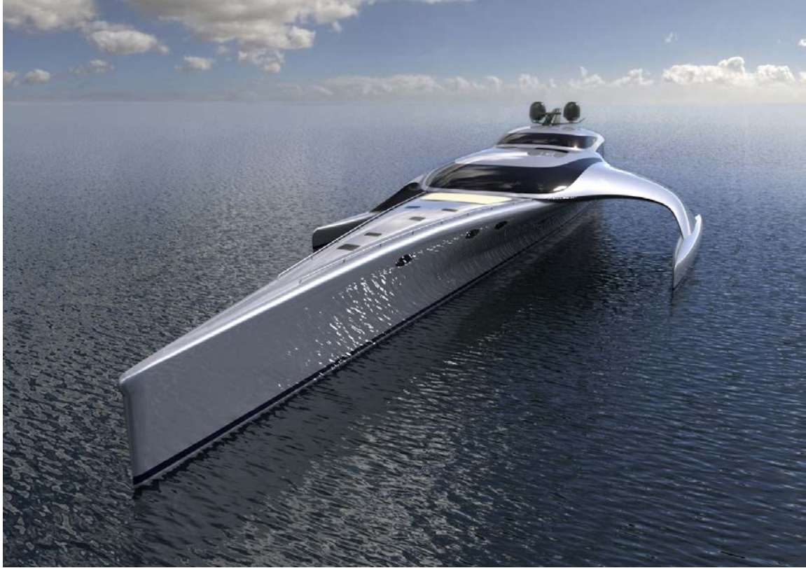
Figure 1. The 42.5-meter trimaran Adastra was recently launched in China. She was designed for exceptionally low fuel consumption, excellent sea keeping qualities and luxurious accommodation. Extensive structural analysis was conducted to account for side slamming, wave impact, and torsional effects of the outrigger riding through waves. The superstructure is carbon fiber with Nomex ® honeycomb core, the hull is glass/Kevlar ® foam sandwich and the interior is light weight oak cabinetry using honeycomb panels. To help reduce weight, virtually every aspect of the boat is custom built. This includes carbon fiber hatches, portlights, ladders and even hinges, which are all built specifically for the vessel.
