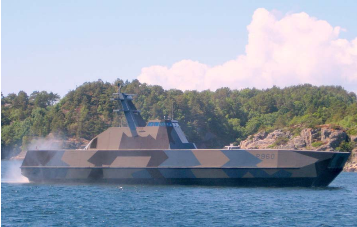
Figure 8. The Skjold is a Littoral Combat Craft (LCC) built by Umoe Mandal in Norway between 1999 through 2006. She has an air-cushioned catamaran hull (surface effect) that relies on lightweight construction for high speed and maneuverability. The ship utilizes flat panels built on a laminating table and joined using secondary bonding methods.
